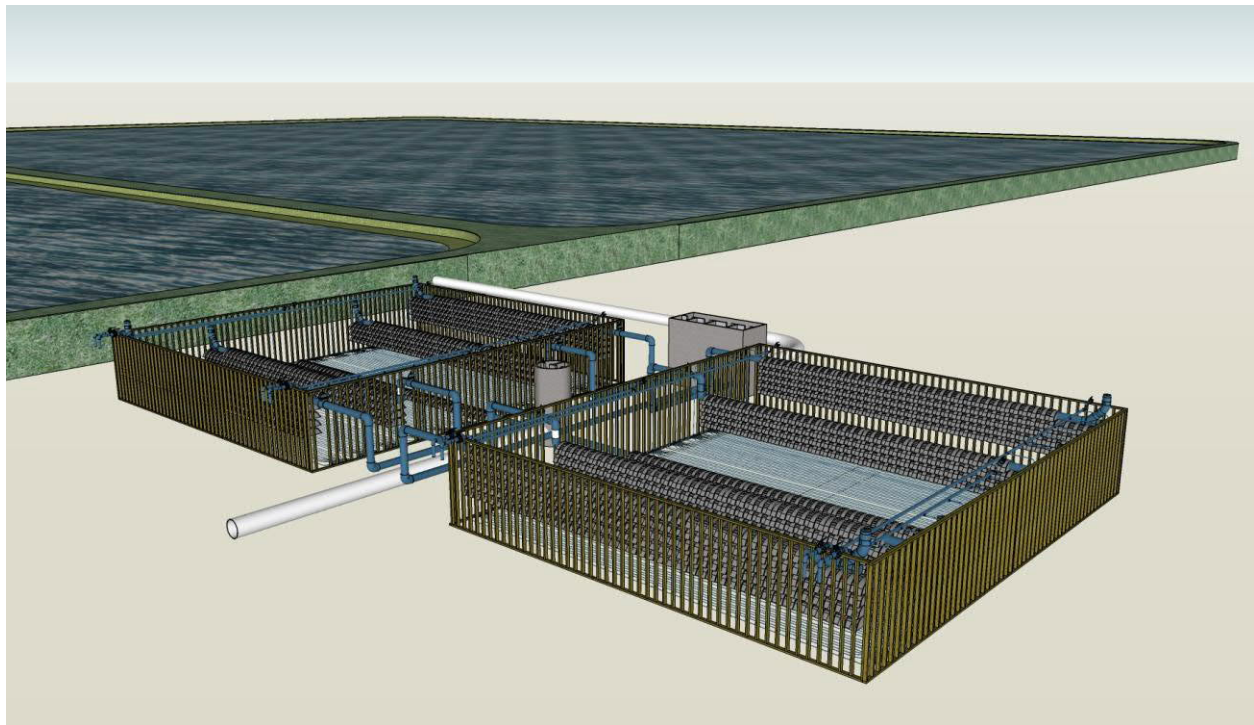
Figure 2: Rendering of the Glencoe, ON SAGR installation (2010) SAGR following aerated lagoon, 1800 m 3 /day
