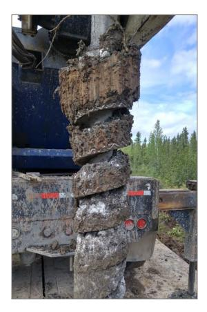
Photo 12: Drilling Borehole 4 at north site. Drill is set up on rig mats. Consistently high ice contents between about 1 and 7 m below ground surface (August 3, 2017).
