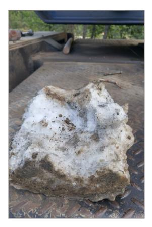
Photo 22: Sample of massive ice lens or layer from Borehole 2 below about 2.3 m. This ice lens has mostly cloudy ice with some clear ice crystals. The lens contains soil inclusions of sand, silt and clay, irregularly distributed in the ice.
