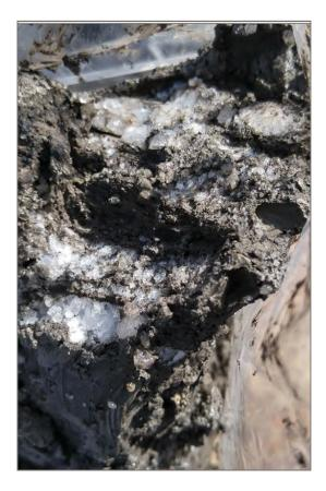
Photo 20: Ice crystals in silty clay till in Borehole 1 of south site, below about 6.4 m below grade.
