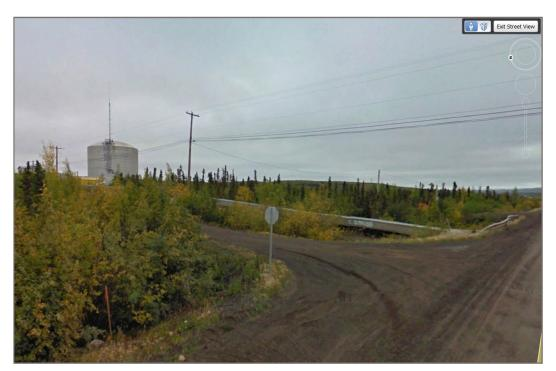
**Photo 8:** Looking southeast at inlet of culvert under Marine Bypass Road, just north of north access road (bottom left of photo, at flagged stake). This culvert would eventually drain surface water from north site. (Photo credit: Google Earth 2017)
