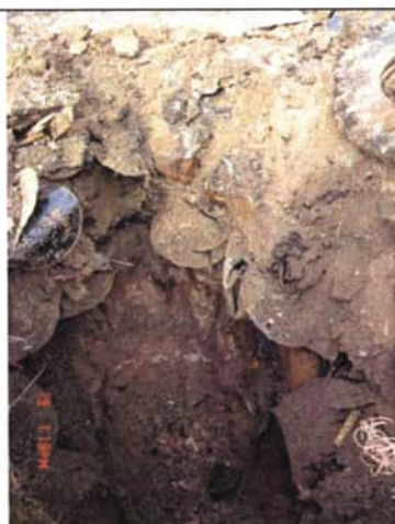
Photo 31 : Debris mainly composed of drums found in 10-TP06-01.
