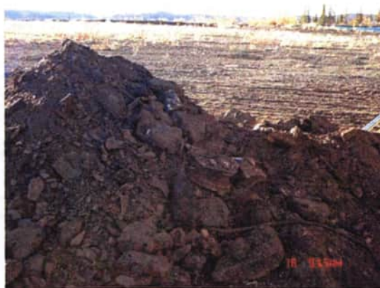
Photo 10 : Debris of all kind found in fill material at 02-TP06-05.
