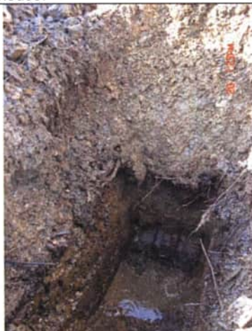
Photo 23 : Presence of water coming from the fill material layer at surface. 08-TP06-03
