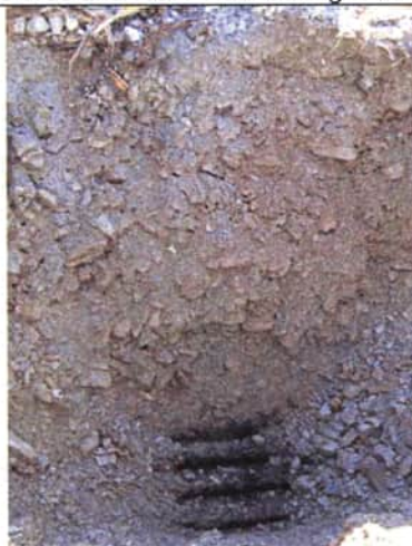
Photo 4 : Typical fill material encountered in test pits located at the former maintenance garage inside footprint. Permafrost at bottom. At 01-TP06-02
