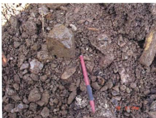
Photo 33 : Ice blocks encountered at 2.9 m below ground surface at 10-TP06-02
