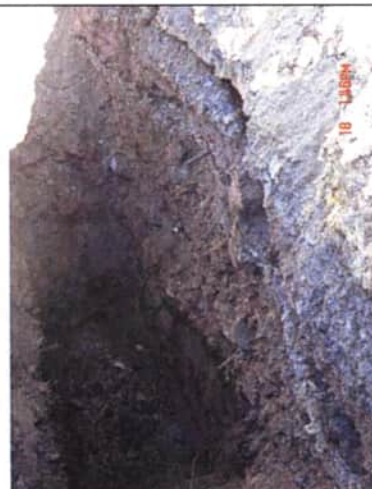
Photo 11 : General stratigraphy observed at FFTA. Fill material at surface, peat layer and native soil. 02-TP06-08
