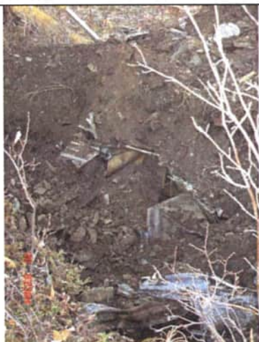
Photo 27 : Debris found at 09-TP06-01. Refusal, pieces are too big, backhoe can not go deeper.
