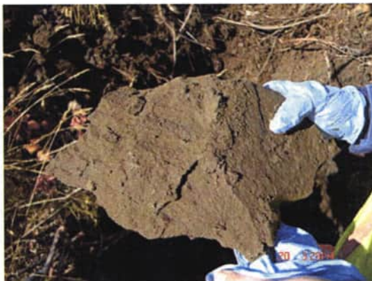
Photo 26 : Sample of permafrost collected from bottom of 08-TP06-07. 1.7 to 1.8 m below ground surface
