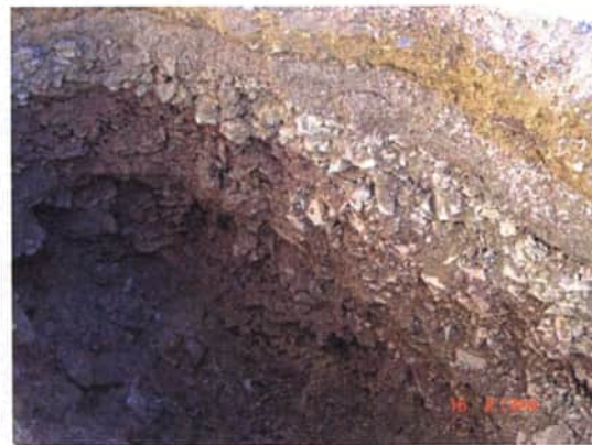
Photo 6 : Typical fill material in former ASTs area, south of former maintenance garage and asphalt road. At 01-TP06-22.
