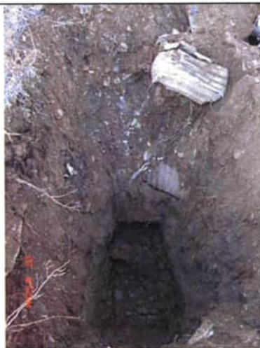
Photo 28 : At 09-TP06-01, because of refusal, extent Test pit toward west to complete it.
