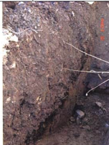
Photo 24 : Typical stratigraphy observed at Shell Lake. Fill material at surface, peat layer and native soil. 08-TP06-05
