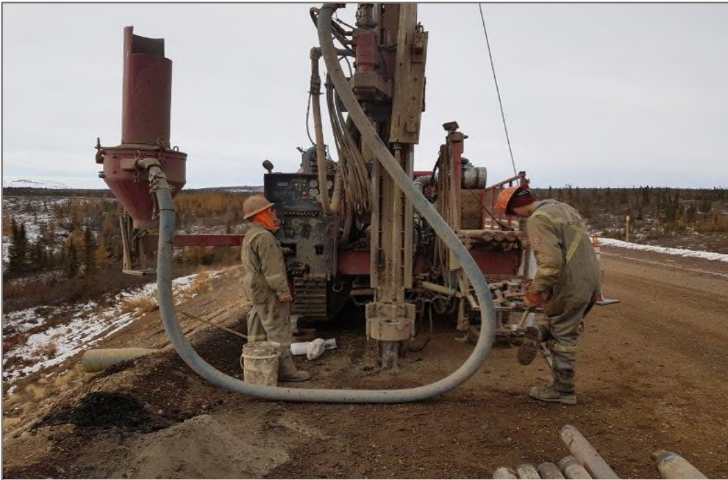
Photo 10: SPT sample collection for BH-04, facing west.
