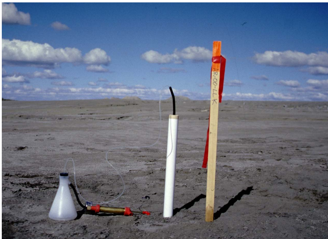
Figure 3.4 – Picture of a sample site with a lysimeter. Lysimeters were placed in the ground about 10 – 20 cm above the ice layer and were purged three times before any analytical samples were taken. The flask and vacuum pump used to remove the water samples from the lysimeter can be seen on the left of the photo.
