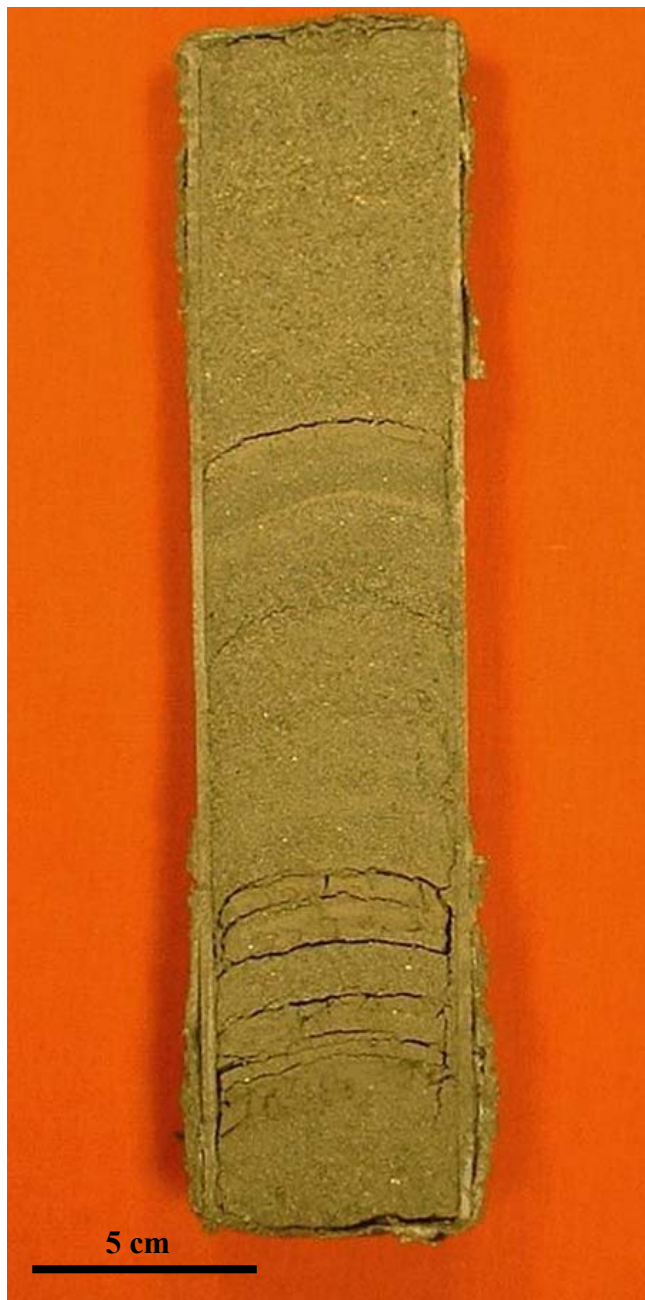
Figure 5.15: Image of processed kimberlite fines core sample. Note the lack of obvious reaction fronts and iron-oxide staining. This image is a very good representation of all processed fines core samples collected for this investigation. The coarse and fine layers evident in this image are caused by the differential settling of coarse and fine material depending on the distance from the process plant discharge spigot.
