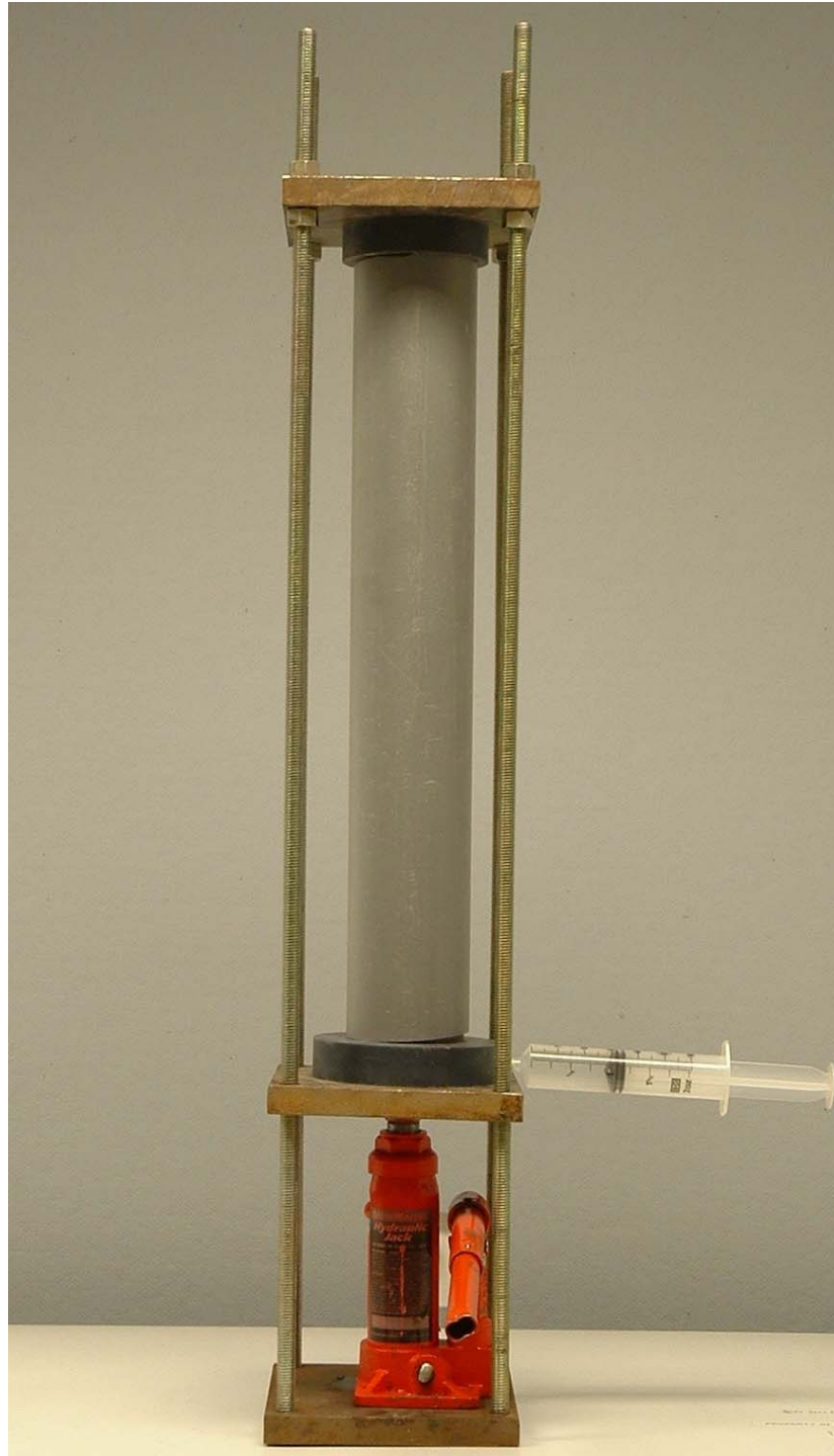
Figure 3.6: Image of assembled pore-water squeezer used in this investigation. The squeezer is approximately 91 cm tall. The syringe on the right hand side of the squeezer has a 60 mL capacity.
