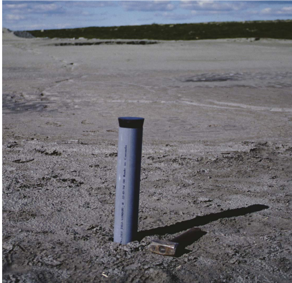
Figure 3.7: Picture showing how core samples of the LLCF kimberlite fines were collected. A PVC pipe was pushed or hammered into the ground and then a rubber stopper was fit into the top end of the pipe to create a partial vacuum. The pipe was then pulled out of the ground and sealed at both ends with laboratory film and duct tape.
