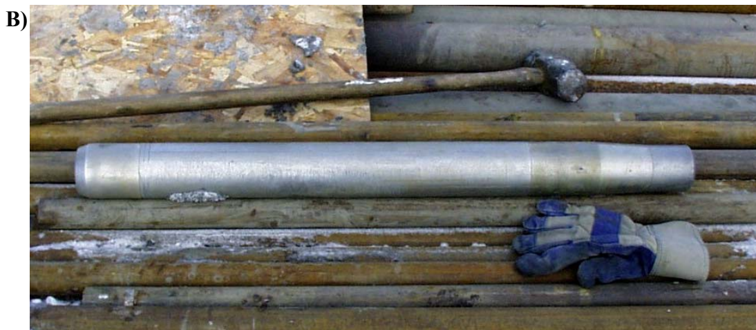
Figure 1.9: A) CRREL barrel used to sample the LLCF fines during the winter 2001 drilling program. Core samples produced are approximately 600 cm in length and 7.6 cm in diameter. B) Split spoon sampler used in the winter 2001 drilling program. Note that the bottom of the sampler is on the left of the photo. This sampler was pounded into the ground using a drop hammer attached to the drill head. The core samples were collected in a cellulose acetate butyrate sleeve that was inserted into the split spoon before it was driven into the ground. Dimensions of the core collected with this sampler are 6.4 cm by 600 cm.
