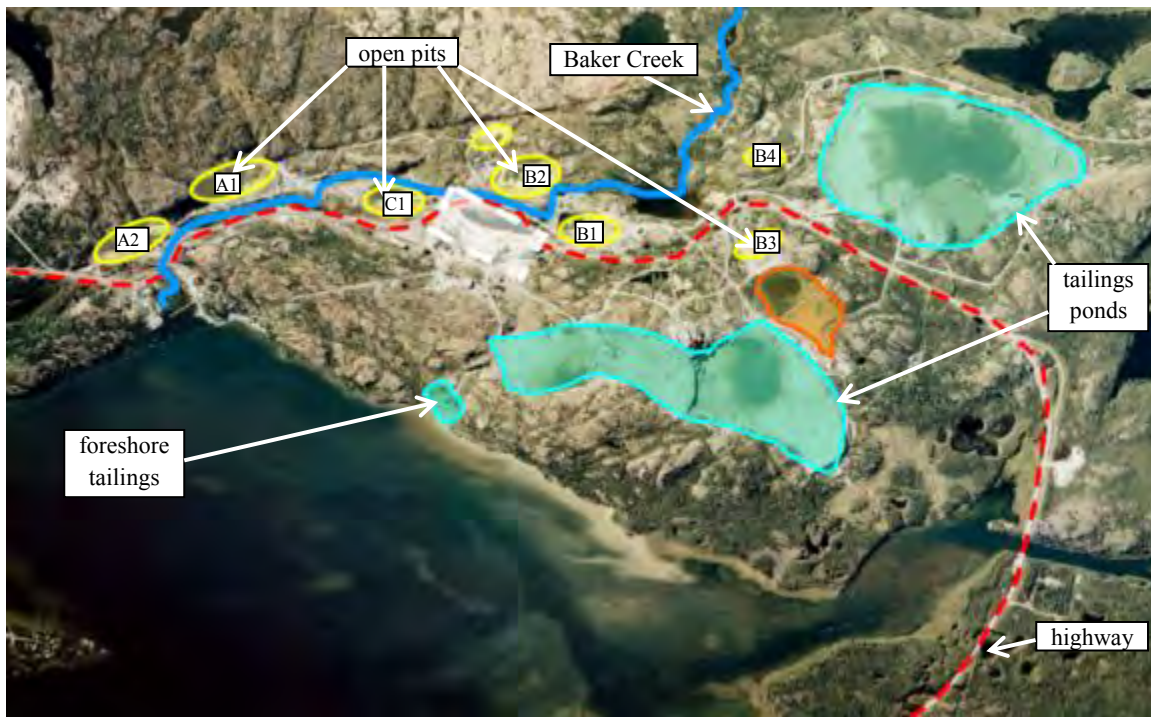
Figure 3. Locations of open pits and tailings ponds [Modified from PR#348 p31]
