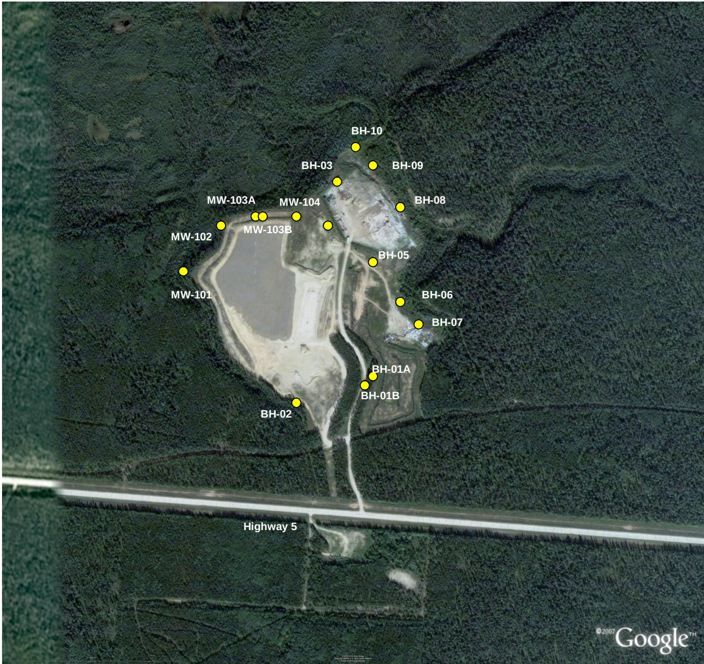
Figure 8 Plan Showing Groundwater Monitoring Wells
