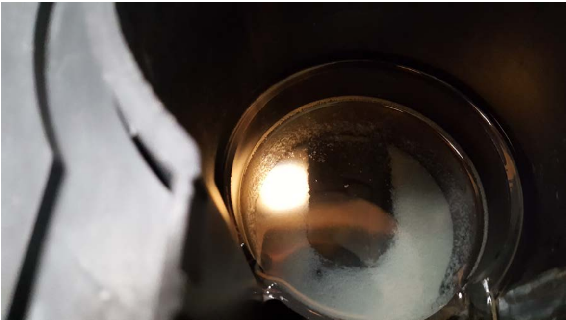
Photo 6: Floc inside turbidity meter after filter
