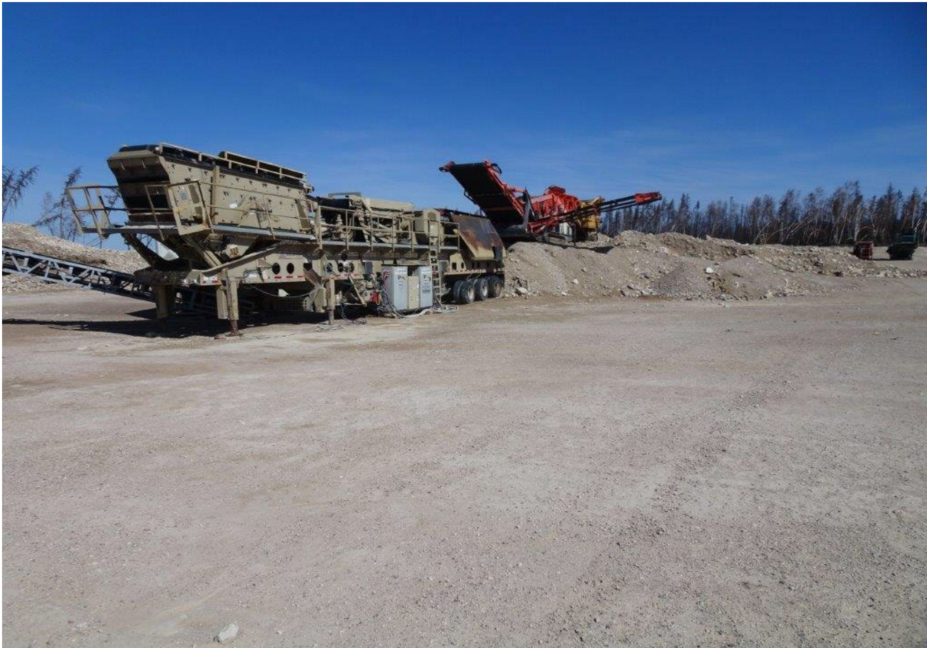
Figure 8 Generator trailer powering the crushing machines at the northeast portion of the quarry.
