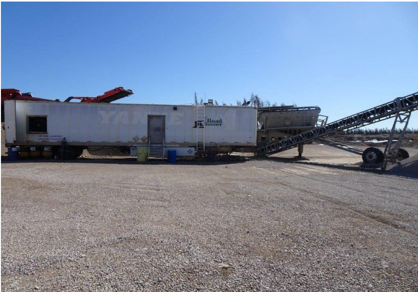
Figure 8 Generator trailer powering the crushing machines at the northeast portion of the quarry.
