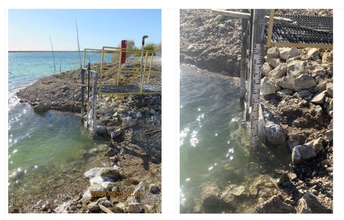
Photograph 25: Main Pond Water Level Gauge at Culvert Intake to Polishing Pond, 22 September 2020
