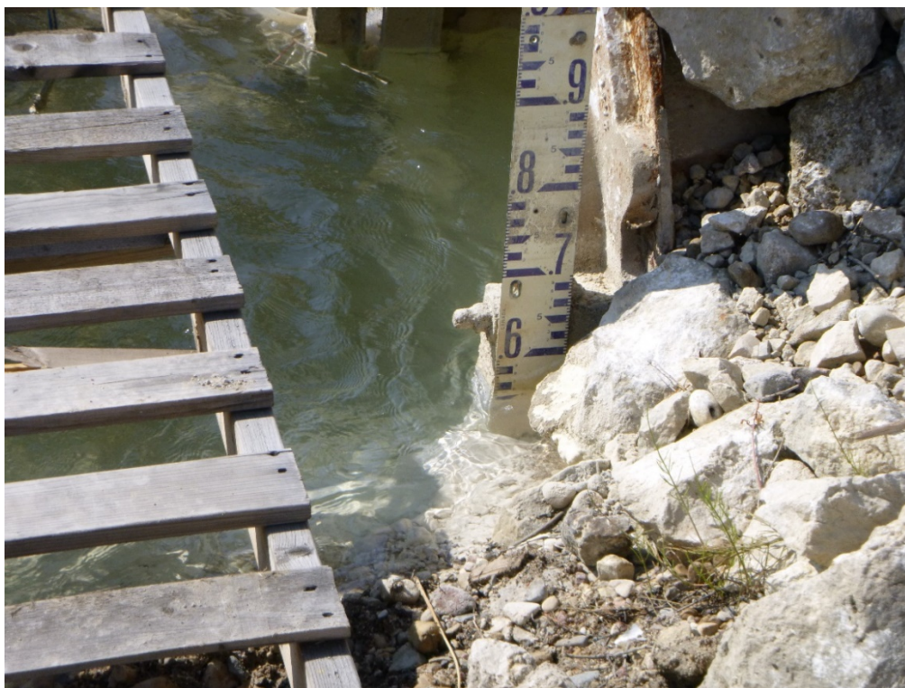
Photograph 19: Main Pond Water Level Gauge at Culvert Intake to Polishing Pond (Elevation 200.558 m), 12 August 2019
