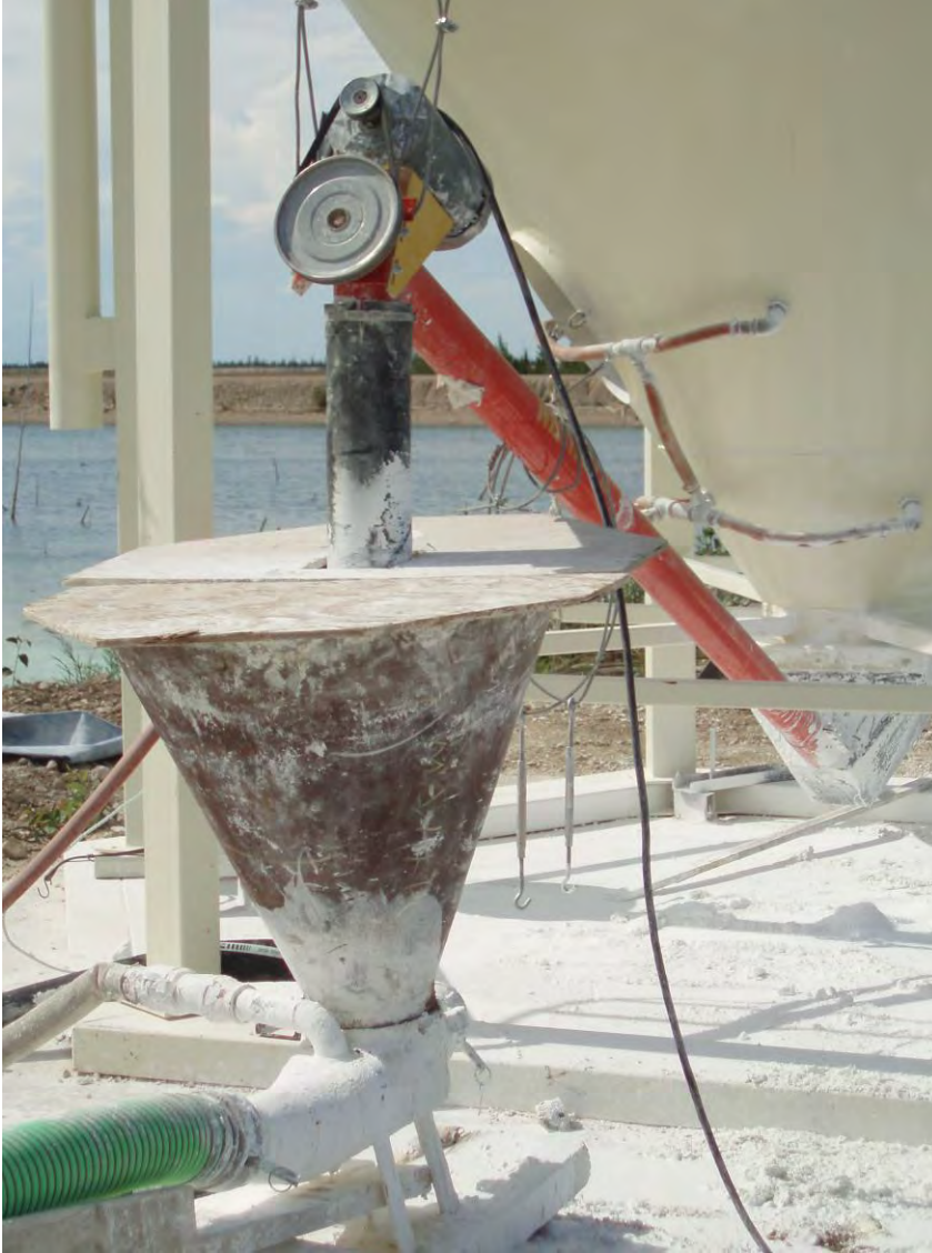
Lime Silo, Auger and Jet Mixer July 2007
