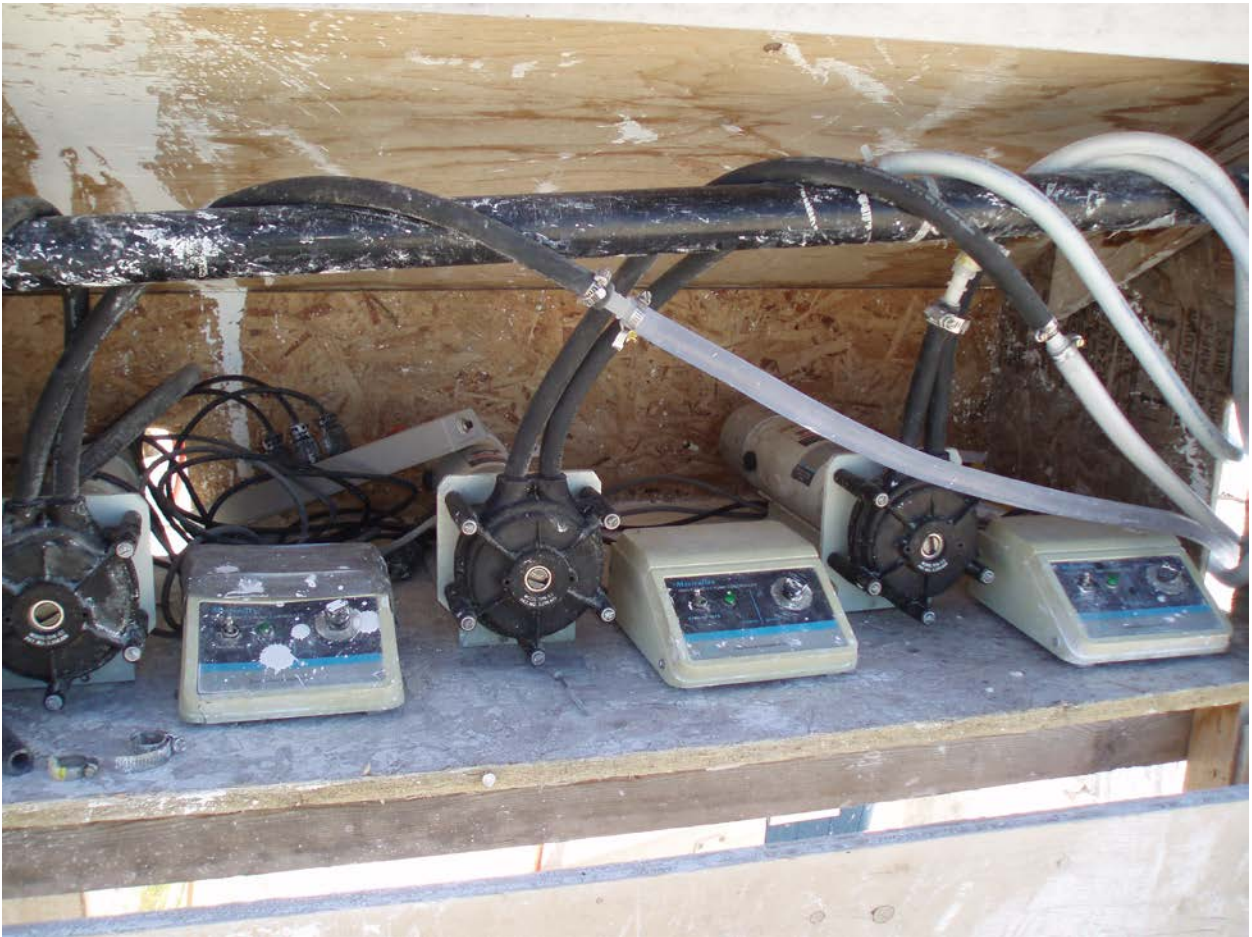
Peristaltic Pumps set up inside the protective stand July 2006
