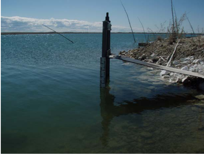
Metric Depth Gauge on Culvert Valve, May 2010
