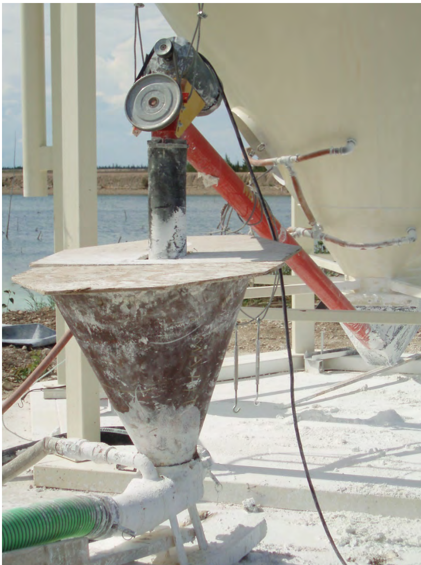
Lime Silo, Auger and Jet Mixer July 2007
