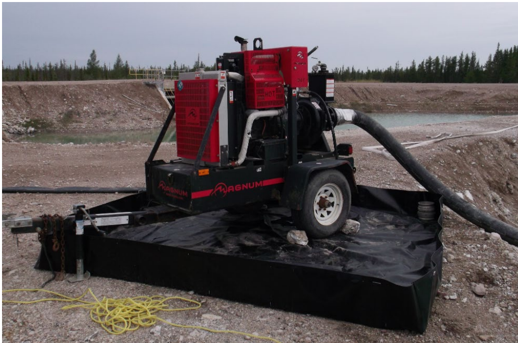
Figure 4.1 Example of Secondary Containment Used with Equipment
