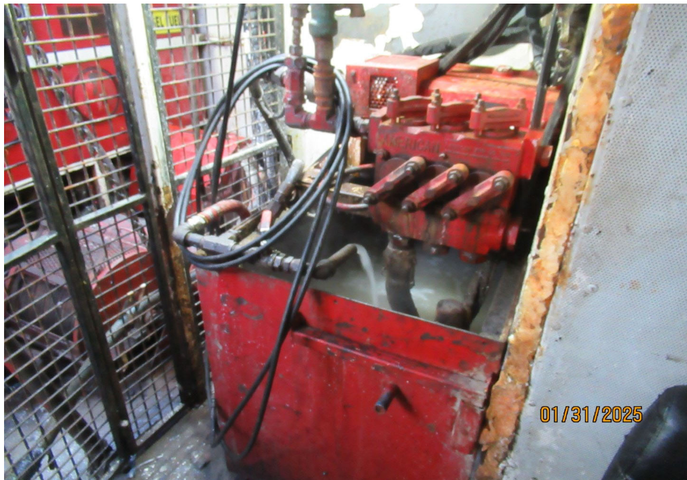
Figure 2 Mud tank inside the drill shack. Water volumes are being minimized since a closed circuit system is in use.
