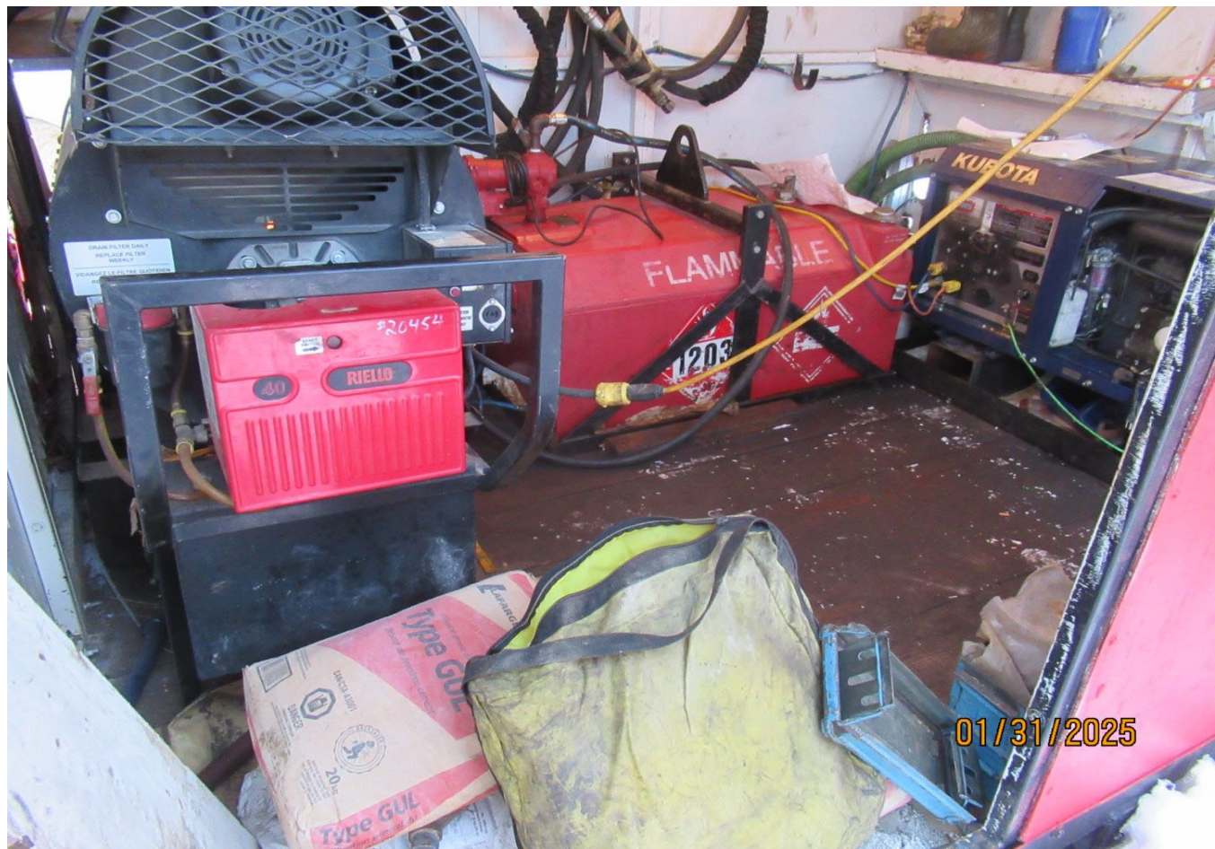
Figure 14 Secondary containment and absorbent matting on a frost fighter.
