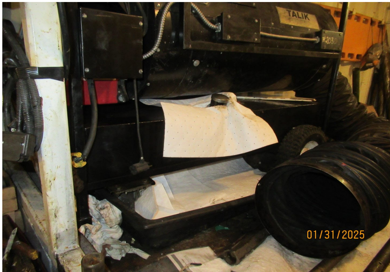
Figure 14 Secondary containment and absorbent matting on a frost fighter.
