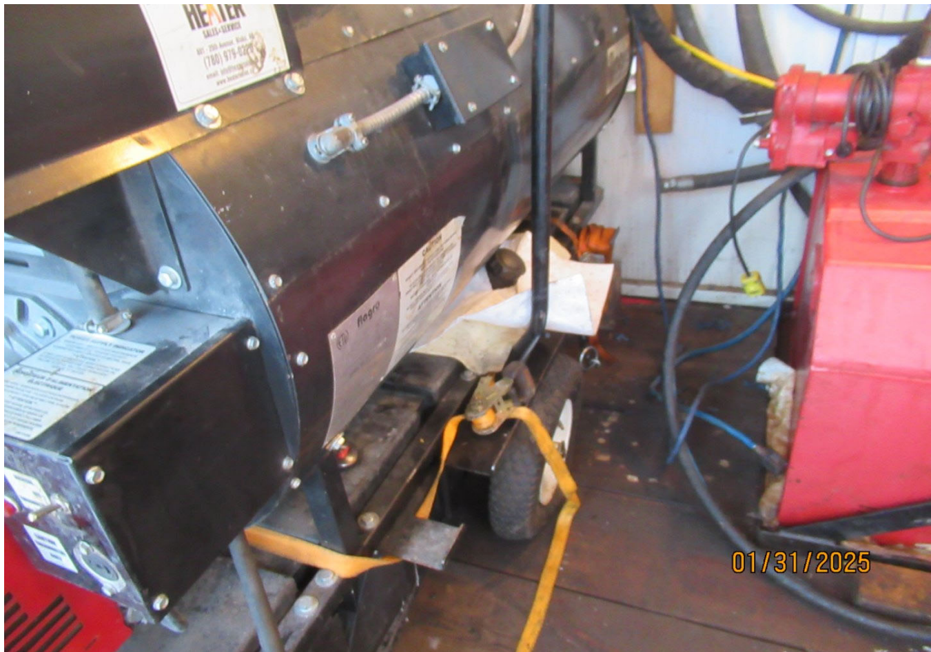
Figure 12 Hydrocarbon absorbent matting is present on all ancillary equipment fuel spouts.
