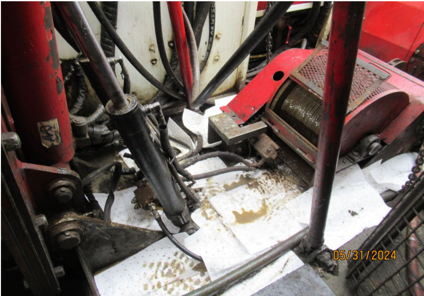
Figure 6 Secondary containment tray below the power pack of the drill.
