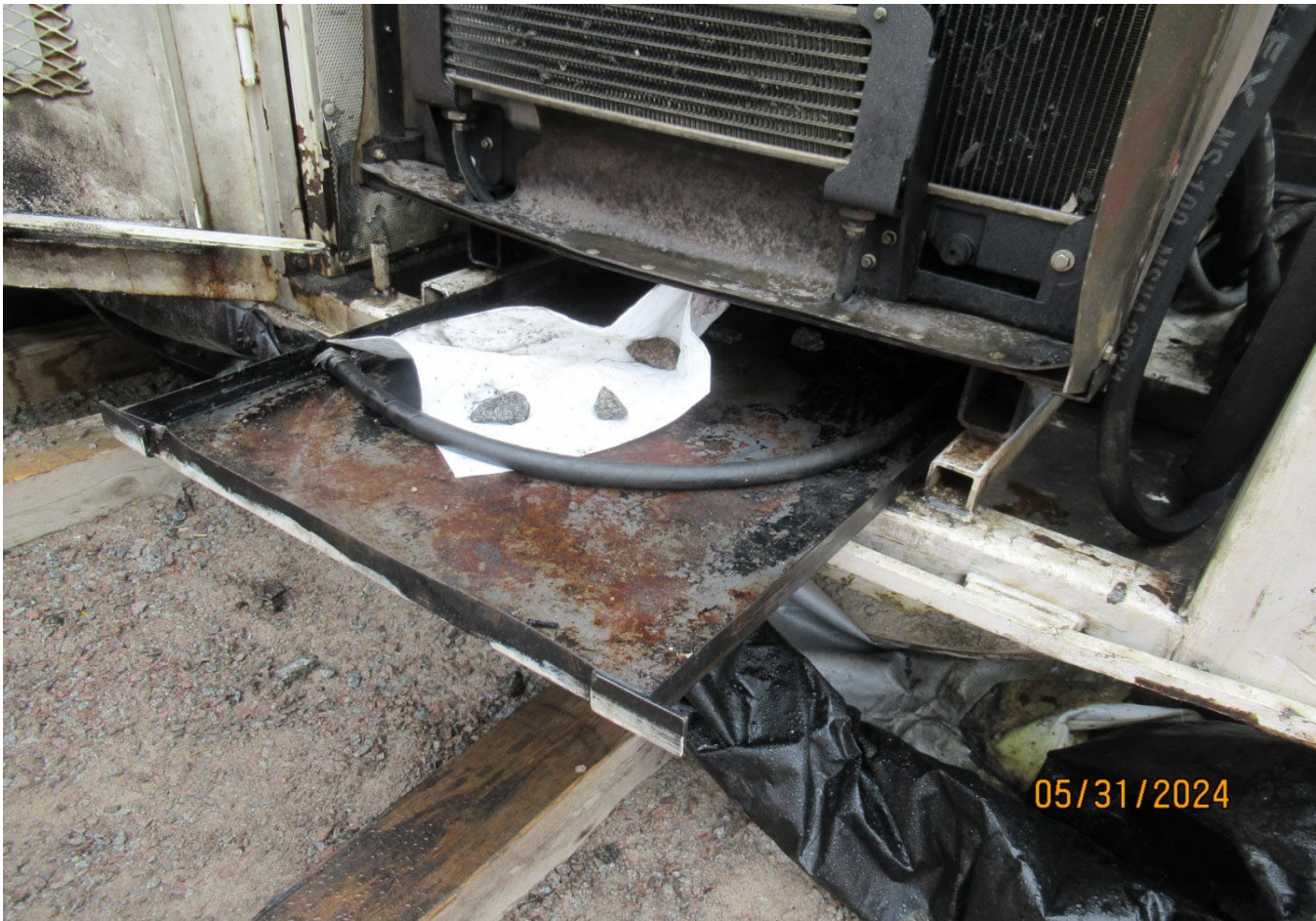
Figure 6 Secondary containment tray below the power pack of the drill.
