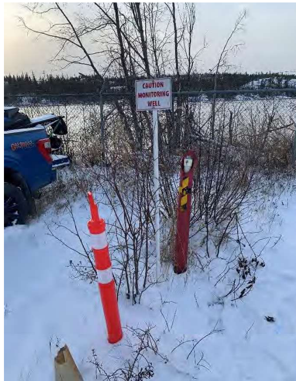
Photograph 6: JF01-03 . Well blocked on the inside. Needs inspection for repair or decommission. Well not sampled. Photograph was taken October 25, 2023.
