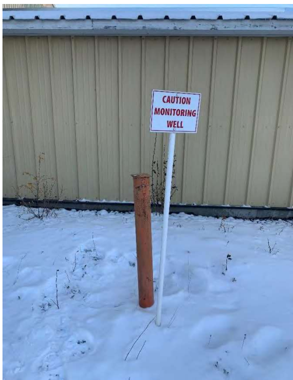
Photograph 18: MW-10 . Appears to be in proper working condition. Hydrocarbon sheen observed during purging and sampling. Well sample collected. Photograph taken on October 25, 2023.
