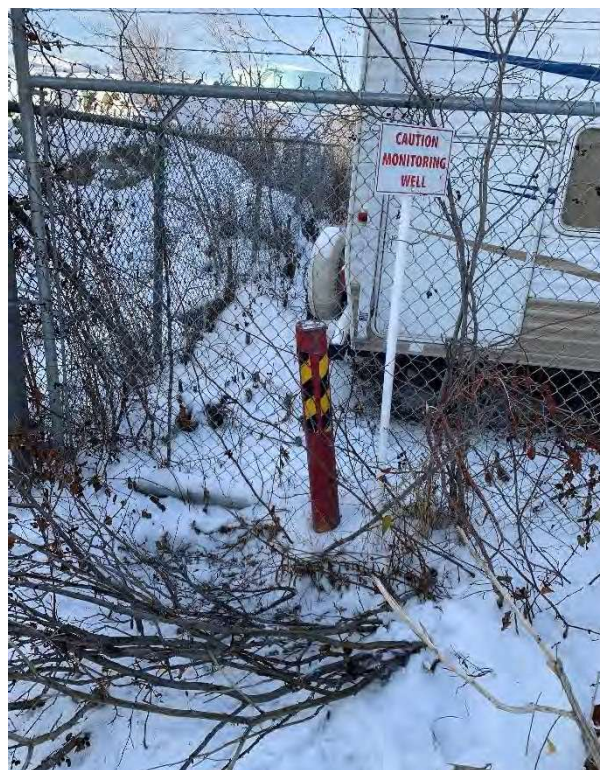
Photograph 4: JF01-01 . Well not horizontal. Appears to be in proper working condition. Hydrocarbon sheen observed during purging and sampling. Well sample collected. Photograph was taken October 25, 2023
