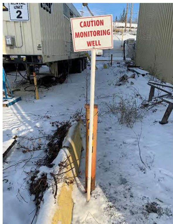
Photograph 16: MW-07 . Appears to be in proper working condition. Hydrocarbon odour observed during purging and sampling. Well sample collected. Photographed taken on October 25, 2023
