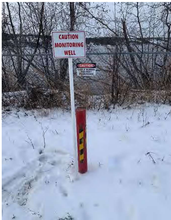
Photograph 8: JF01-05 . Dry well. Insufficient water to sample. Needs inspection for possible repair or decommission. Photograph was taken October 25, 2023.
