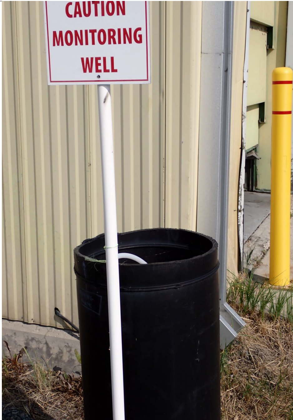
Figure 4 - Groundwater monitoring well without cap
