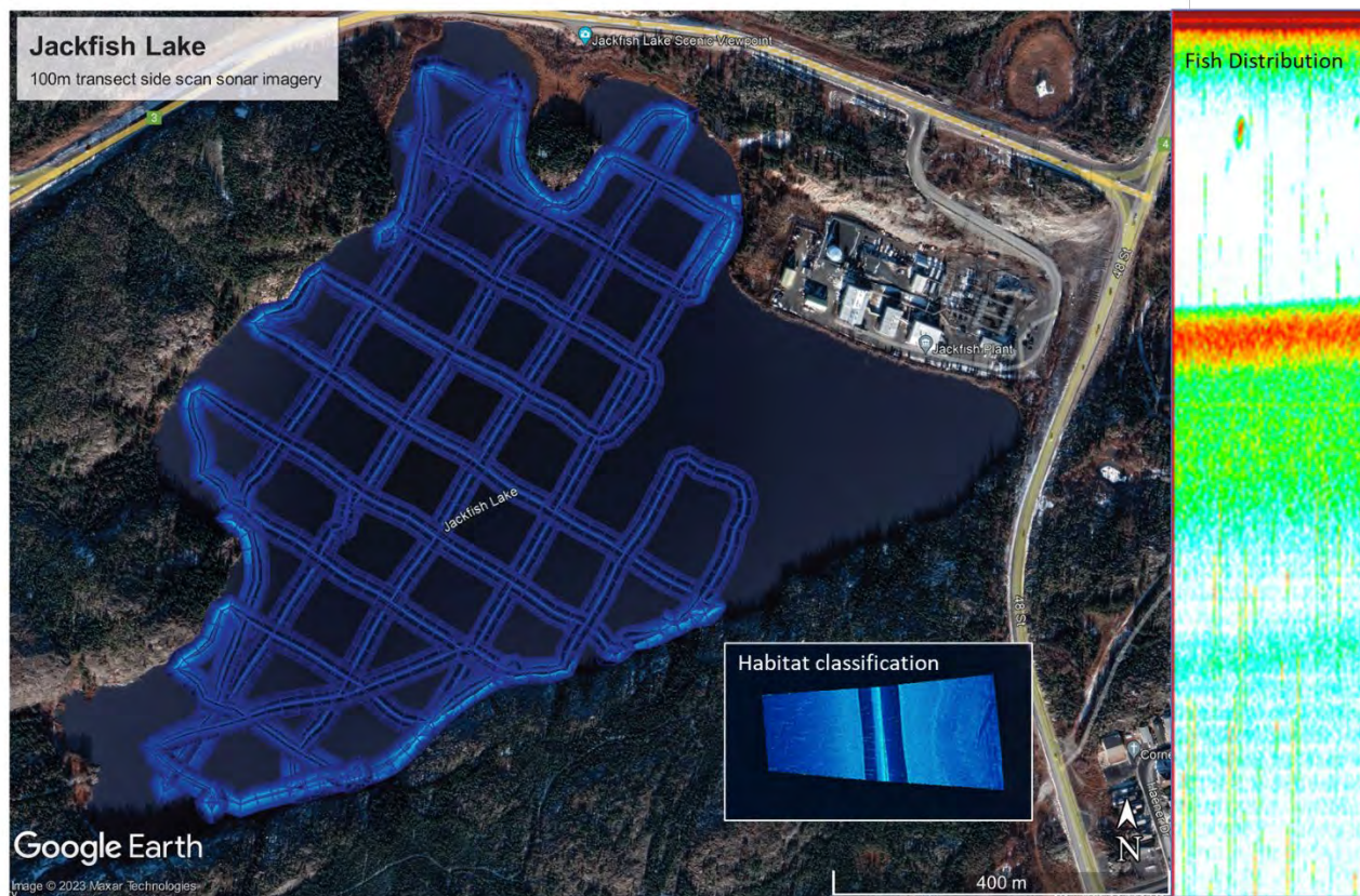
Figure 2.3-2: Example of the Sonar Imagery Evaluated for Habitat Classification (Transect R00037; TileT000) and Fish Distribution (Transect R00039; Tile T475) in Jackfish Lake
