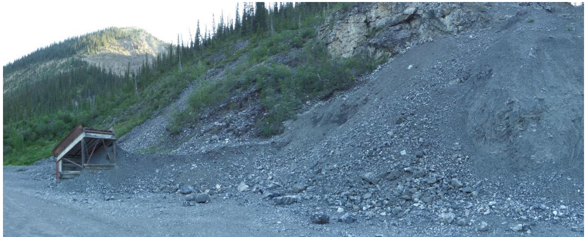
Figure 1: BP2 materials pushed from a higher rock face for screening with a grizzly.
