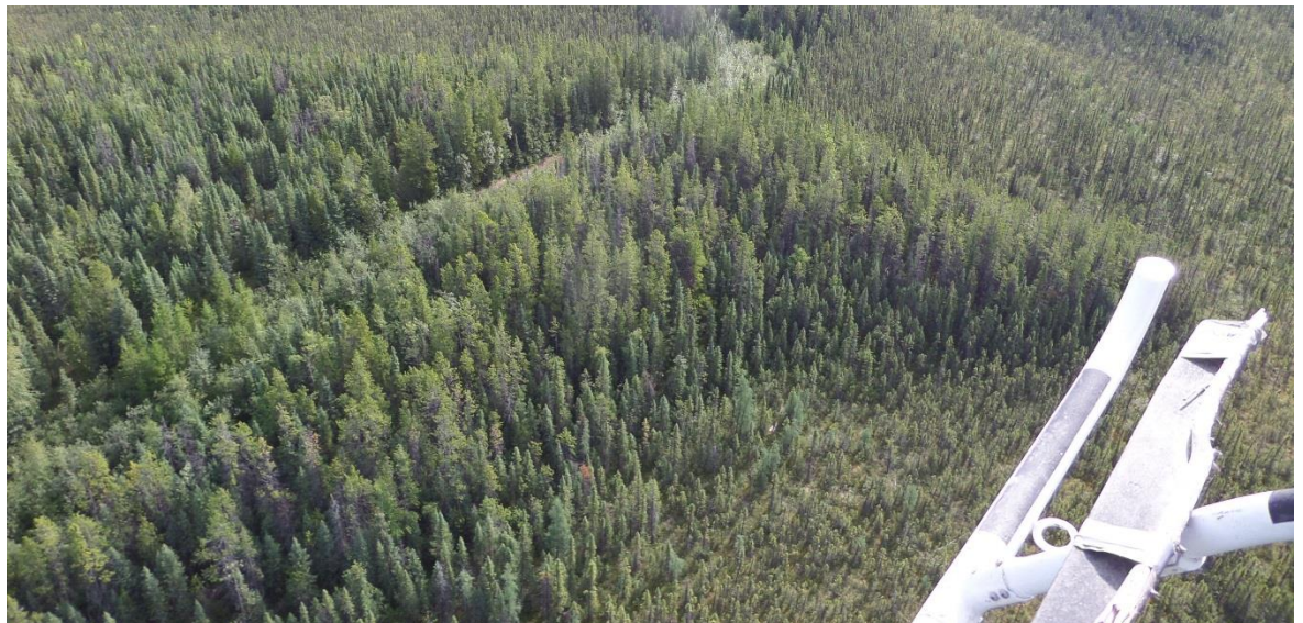
Figure 48: A small ridge of sandy till (BP78) lies under the road route at 78.0 km. The drier material here could be used to construct adjacent overland fills.
