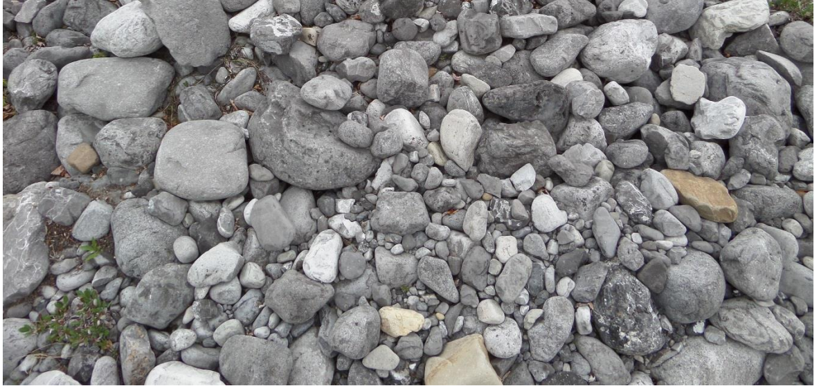
Figure 13: Typical gravel and cobble material available at BP39A. This material consists primarily of Paleozoic carbonate rocks as evidenced by the abundance of fossilized coral fragments throughout the aggregates.
