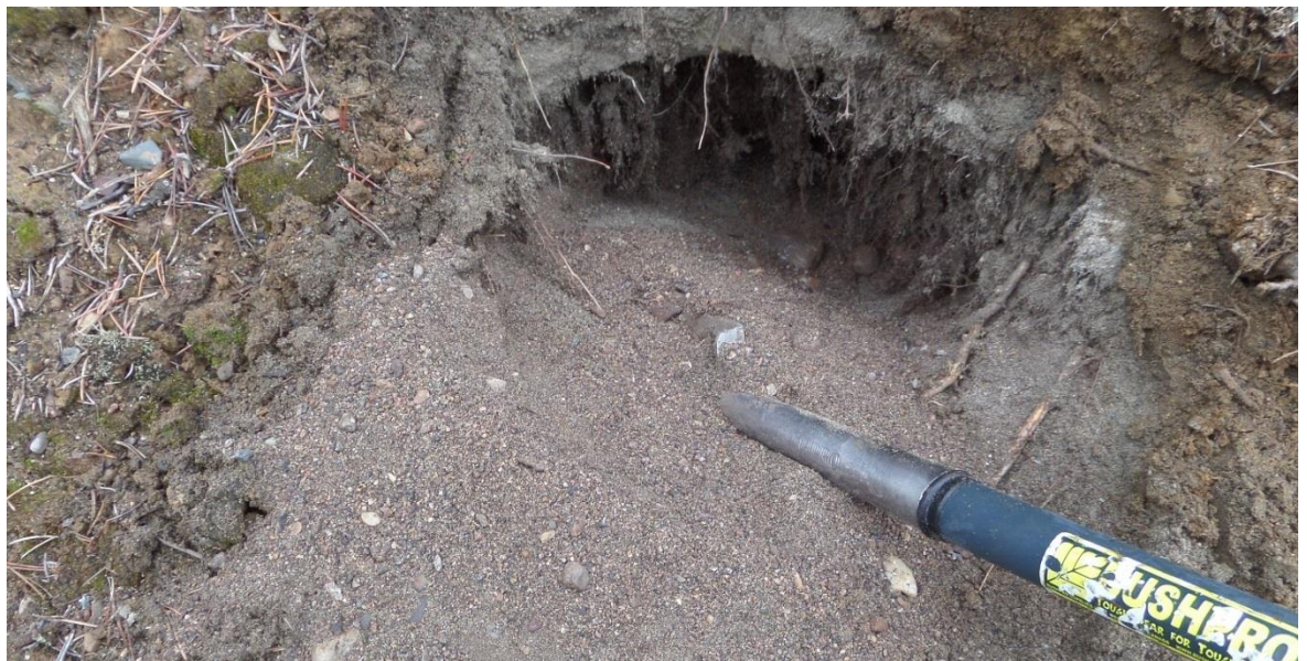
Figure 50: Sand material found in an existing cut slope at 86.35 km. This is some of the cleanest sand noted in the area and could be used for pipe bedding and overland fills.
