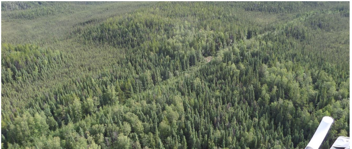
Figure 46: A low ridge of higher sandy till (BP77A) crosses over the road route laterally at 76.7 km. This source of drier material could be used to build some of the overland fills that will be required to cross the wetland.
