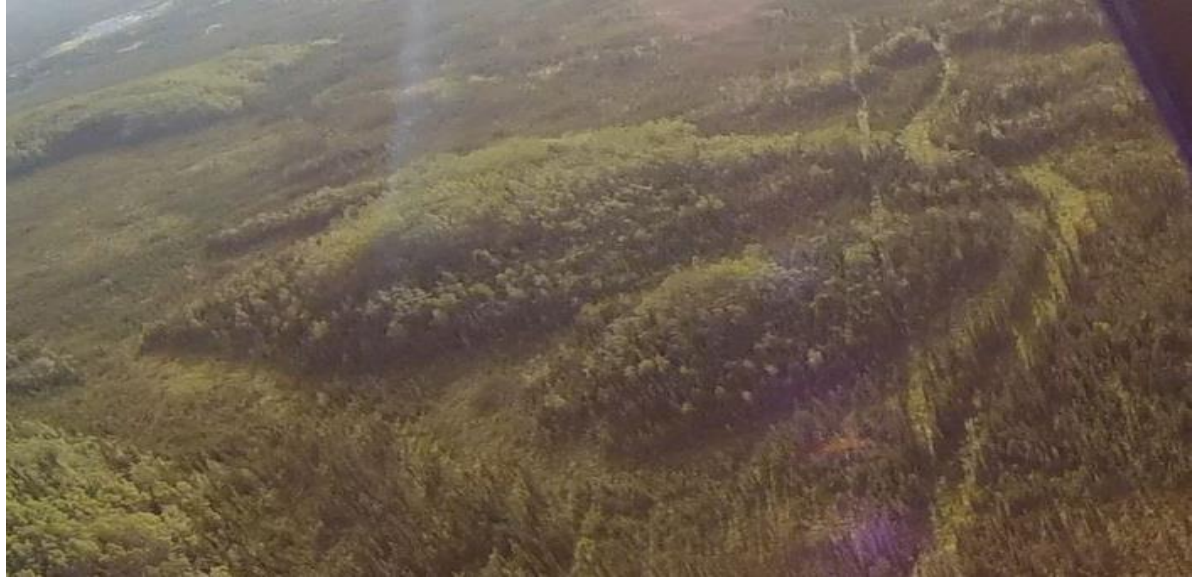
Figure 60: Dry elevated “humps” covered with lodgepole pine and aspen should provide adequate silty clay type material for overland sections.
