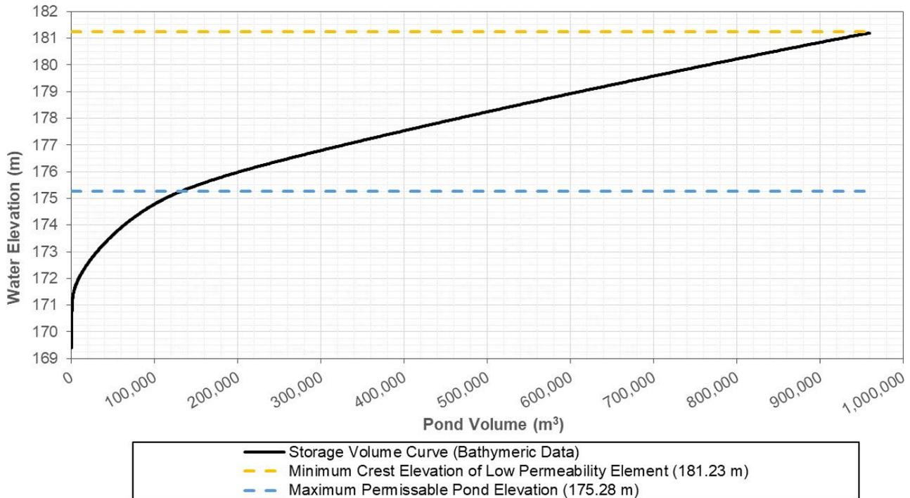
**Figure 8: Water Elevation Versus Storage Volume – North Pond**
