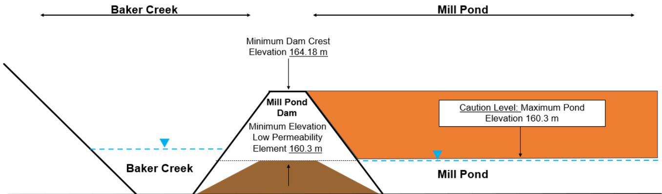
Figure 13: Water and Infrastructure Elevations for Mill Pond Structure and Baker Creek (not to scale)
