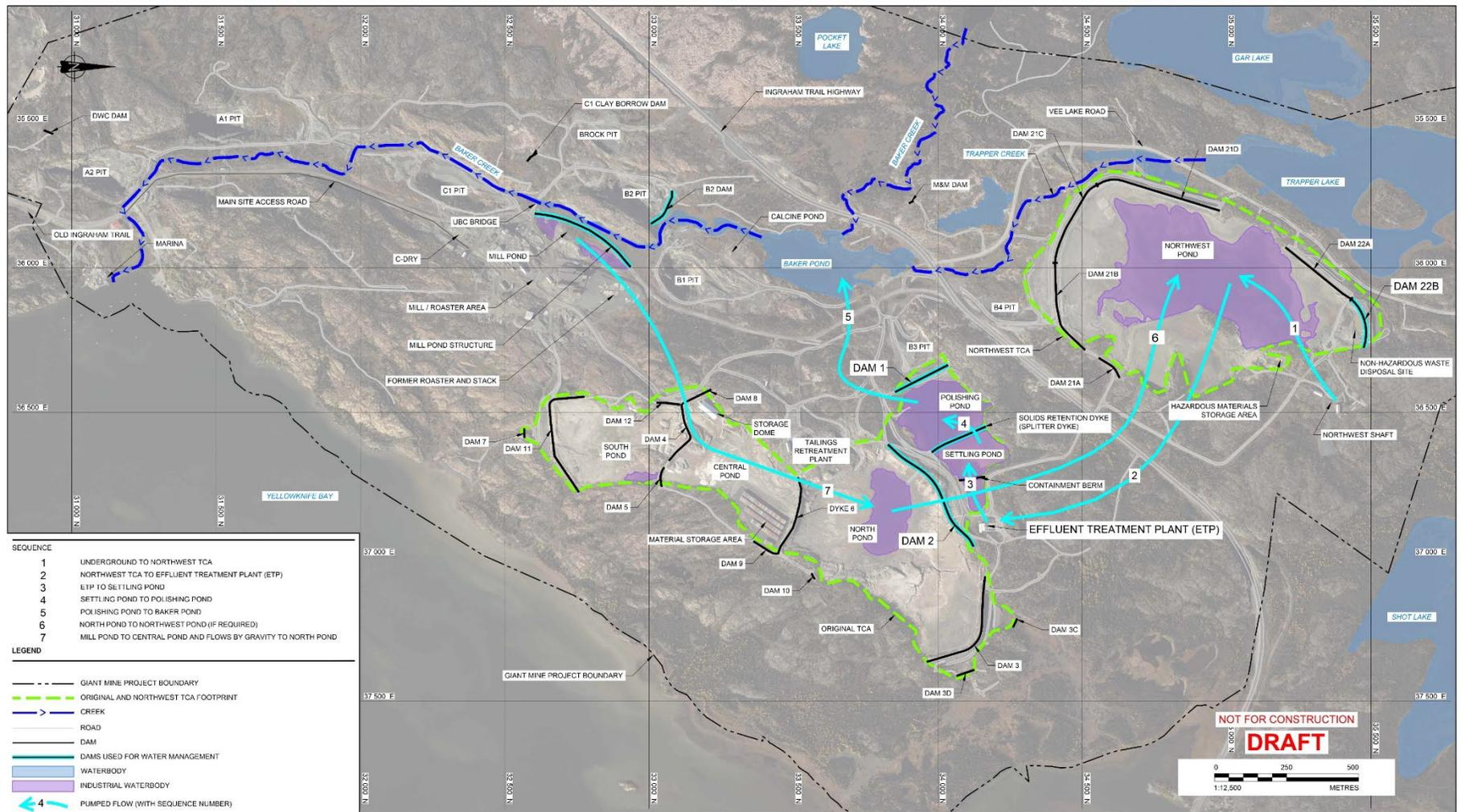
Figure 6: Overview of Water Treatment at Giant Mine
