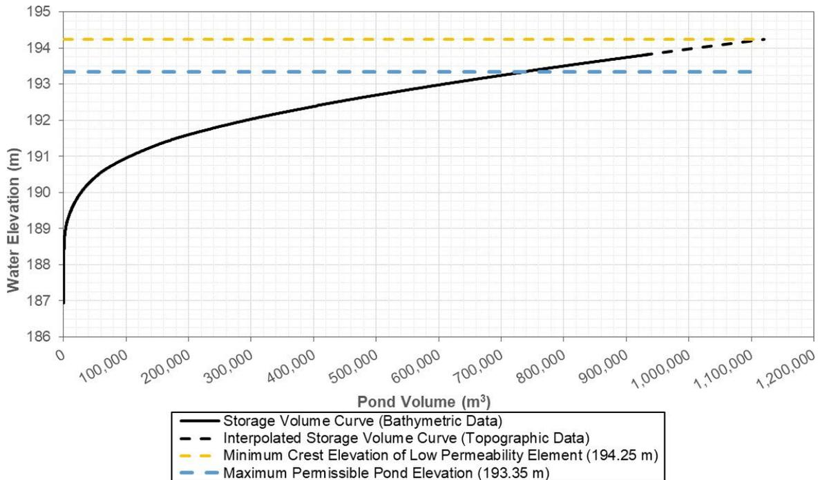
**Figure 7: Water Elevation Versus Storage Volume – Northwest Pond**
