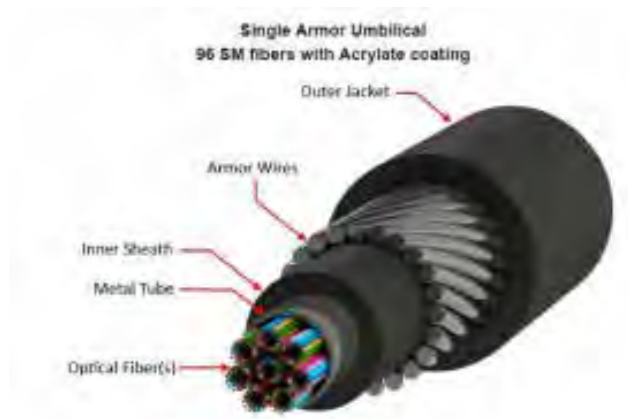
Plate 2-1 Typical Cable Considered for Direct-buried or Surface-laid installation
