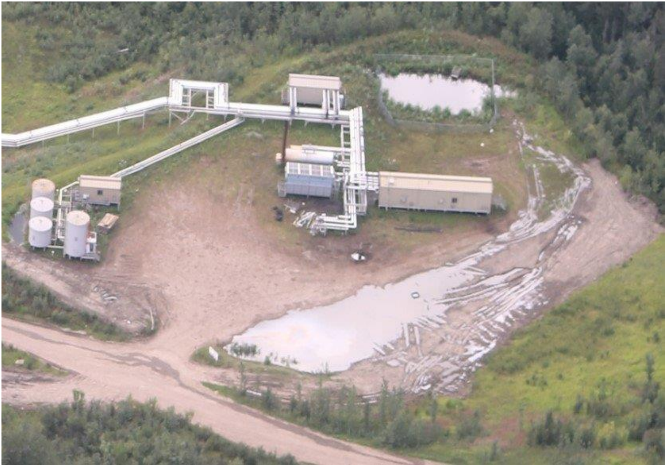
Figure 8 F-25/F-25A- note sump overflowing
