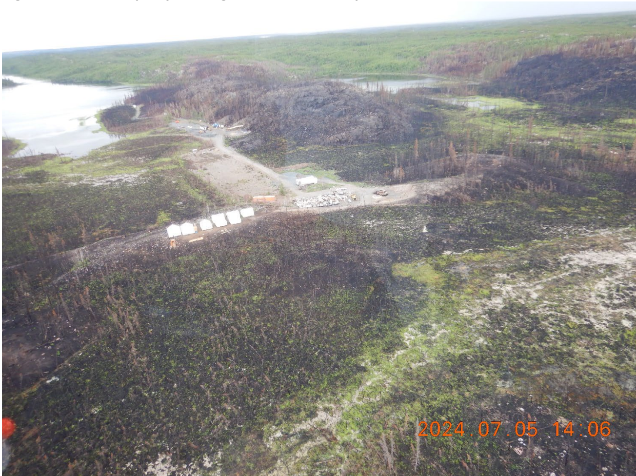
Figure 2 – Mon Property portal, waste rock storage pile and mine water settling pond.
