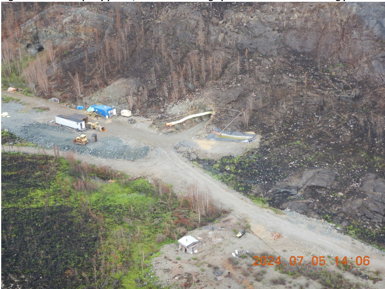
Figure 2 – Mon Property portal, waste rock storage pile and mine water settling pond.
