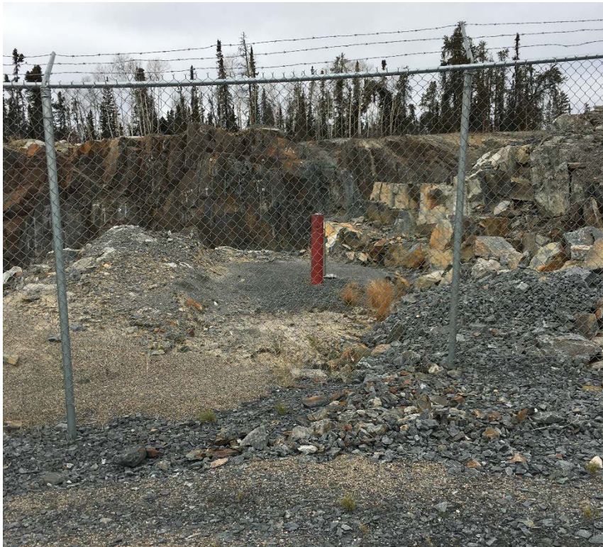
Figure 5-12: Piezometer SP01 shown outside of the perimeter fence, restricting access which has less led to the instrument not being monitored
