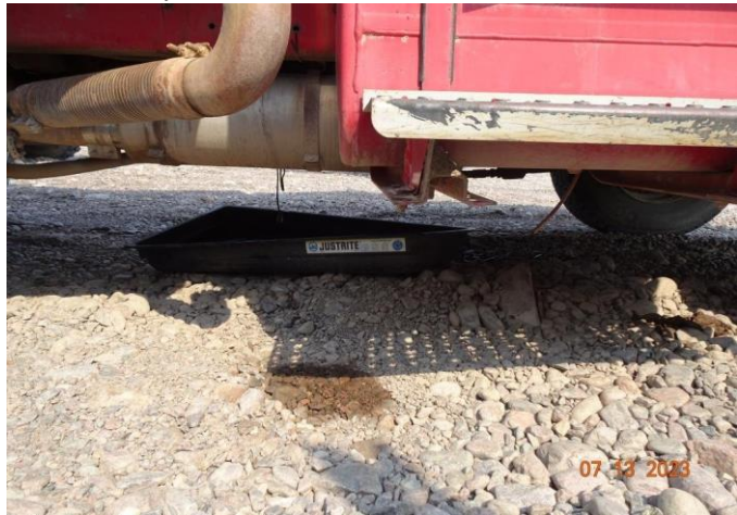
Figure 29 Hydrocarbon staining and drip tray underneath NTPC dump truck #3027.
