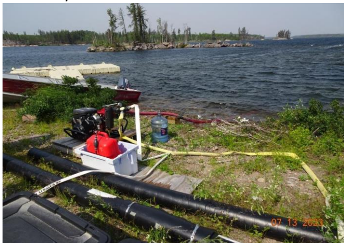
Figure 12 Emergency water pump and 25L jerry can in secondary containment.
