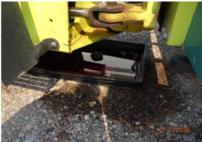
Figure 27 Hydrocarbon staining and full drip tray underneath the AMMANN single drum roller.
