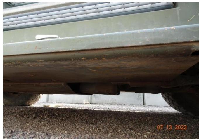
Figure 27 Hydrocarbon staining and full drip tray underneath the AMMANN single drum roller.
