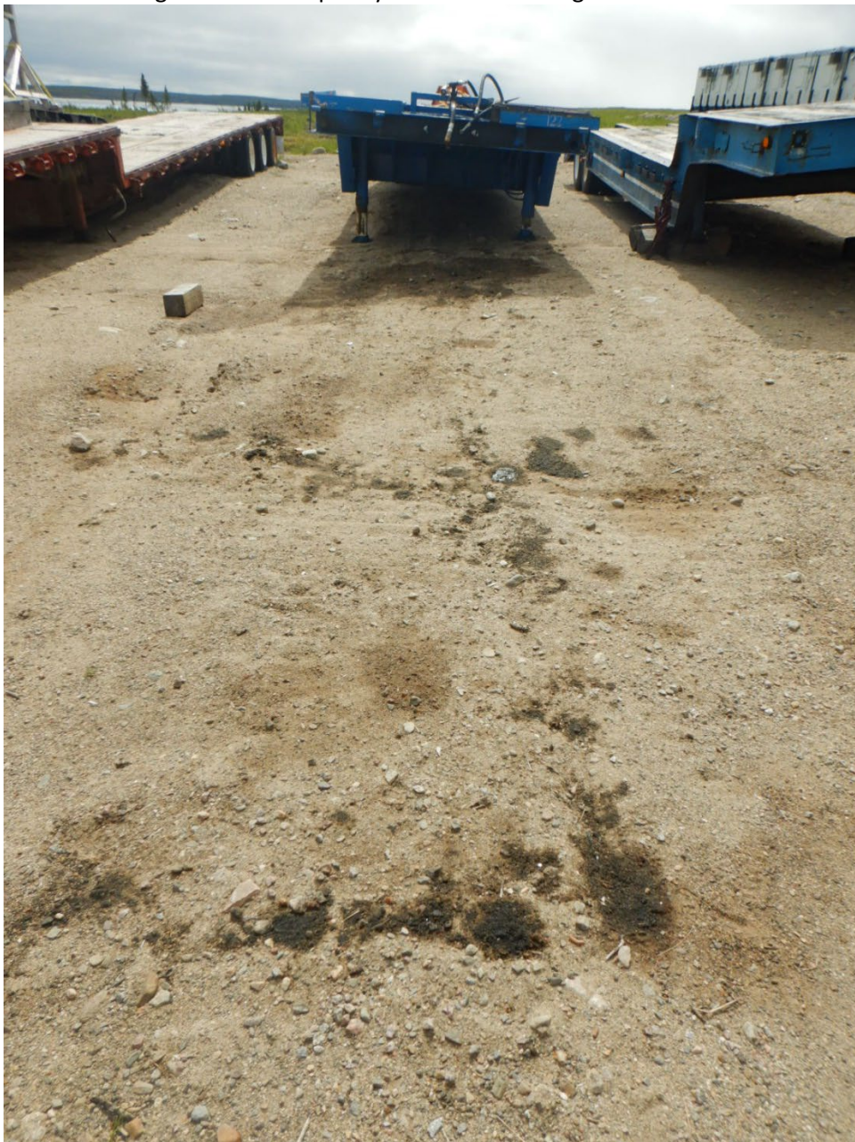
Photo 4 – Margaret Lake Camp – Hydrocarbon staining under and around flatbed (2).
