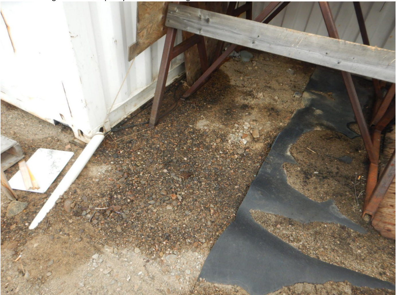
Photo 14 - Margaret Lake Camp – Hydrocarbon staining underneath raised fuel tank.
