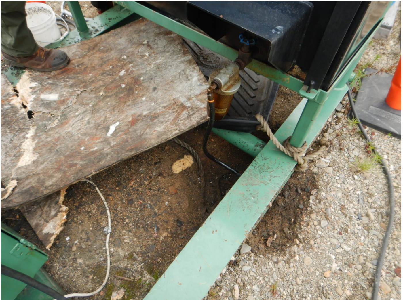
Photo 17 - Margaret Lake Camp – Hydrocarbon staining from a potential fuel line leak.
