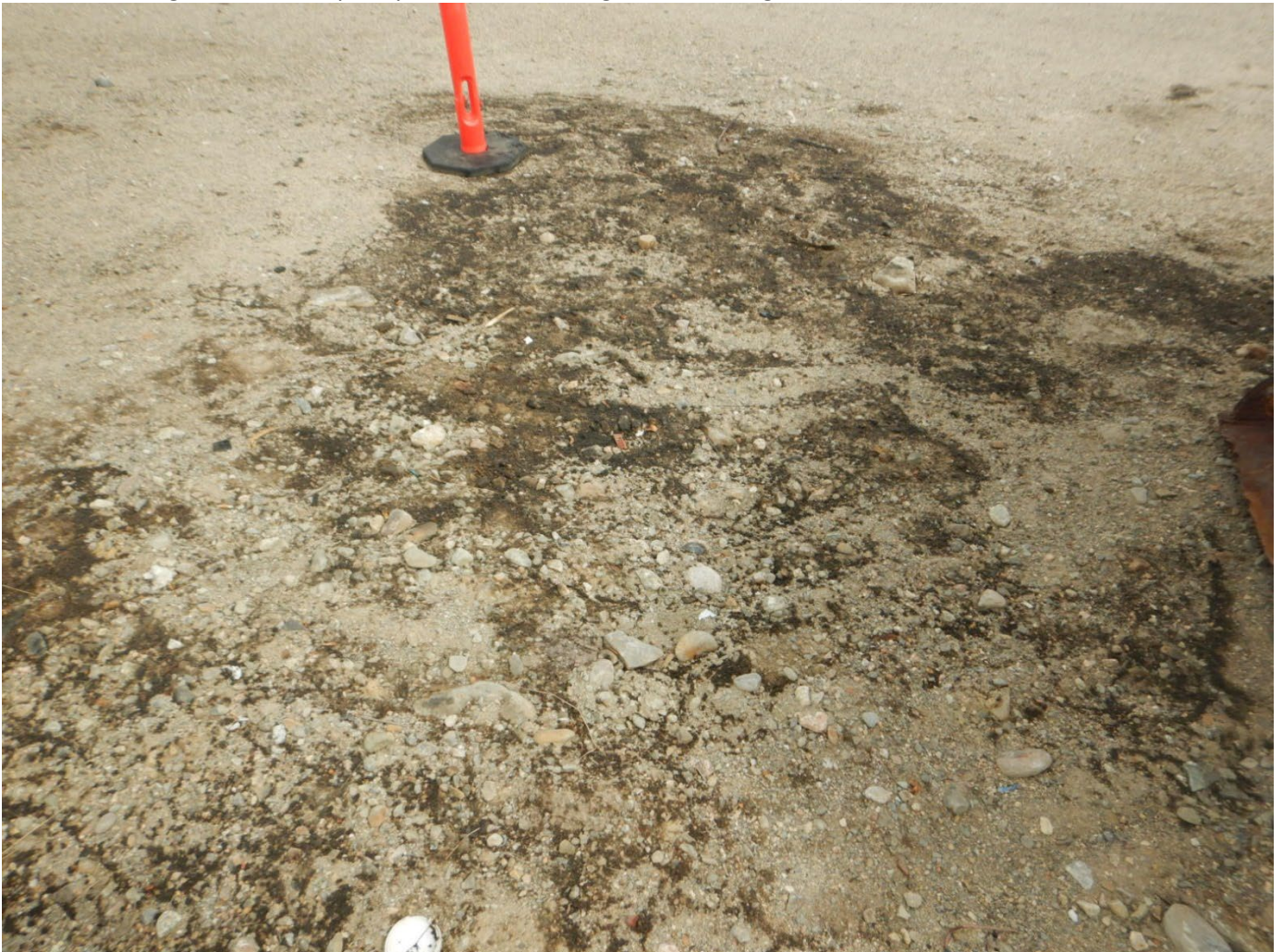
Photo 12 - Margaret Lake Camp – Hydrocarbon staining near refueling area (1).
