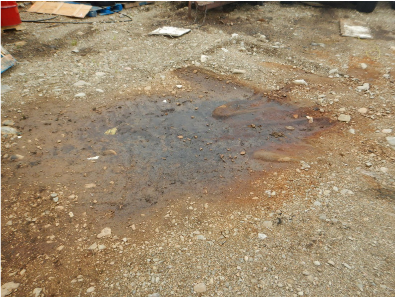
Photo 11 - Margaret Lake Camp – Hydrocarbon staining near staged equipment area.
