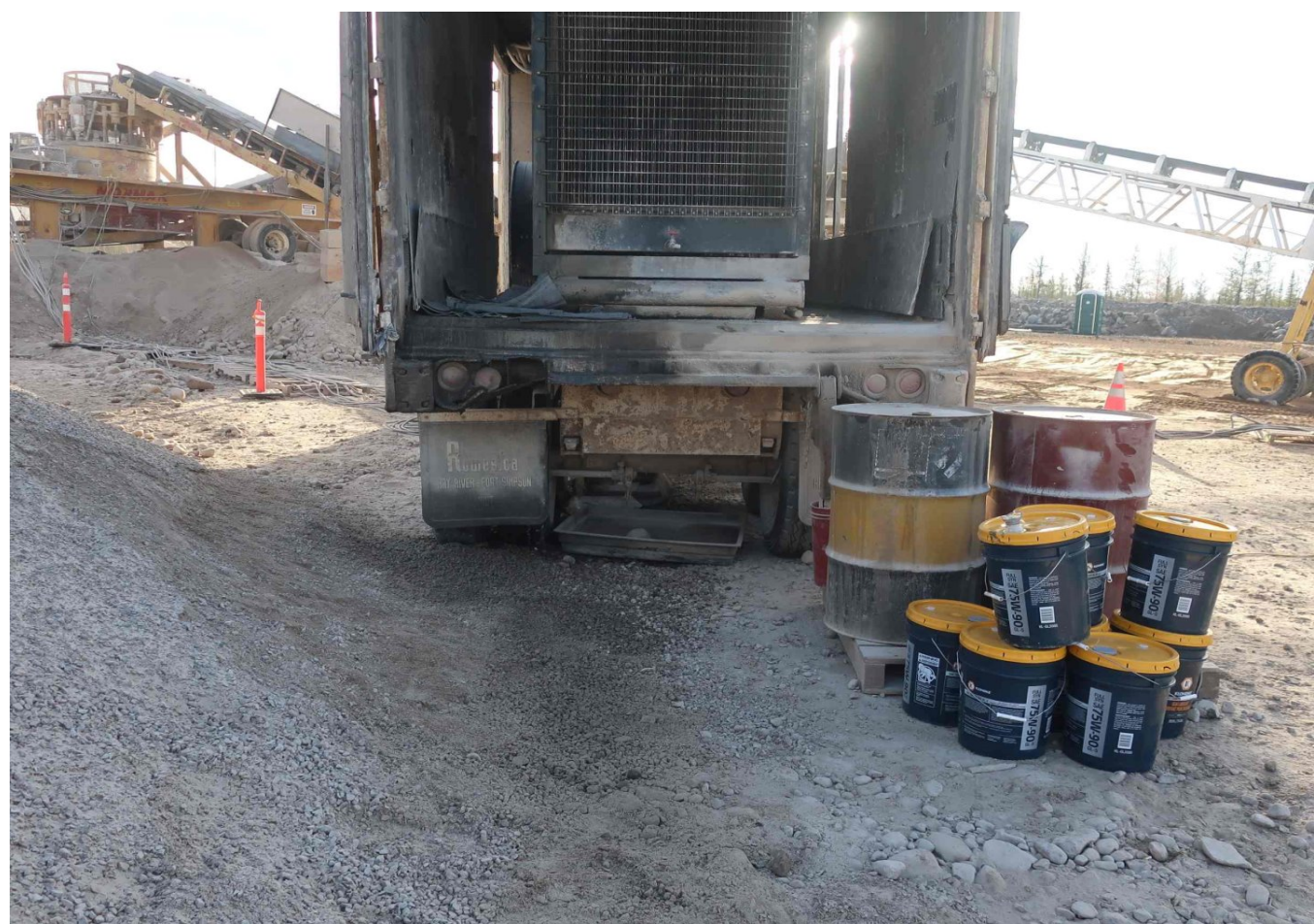
Figure 4 Glycol leaking out the back of the crusher generator trailer.
