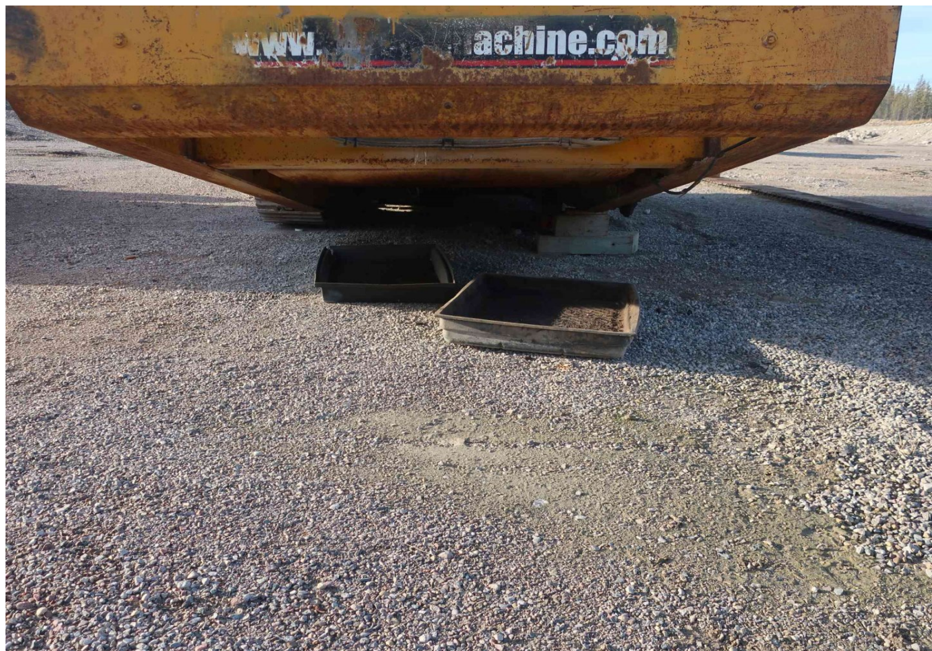
Figure 10 Drip tray in place under crusher stored on the north side of the pit.
