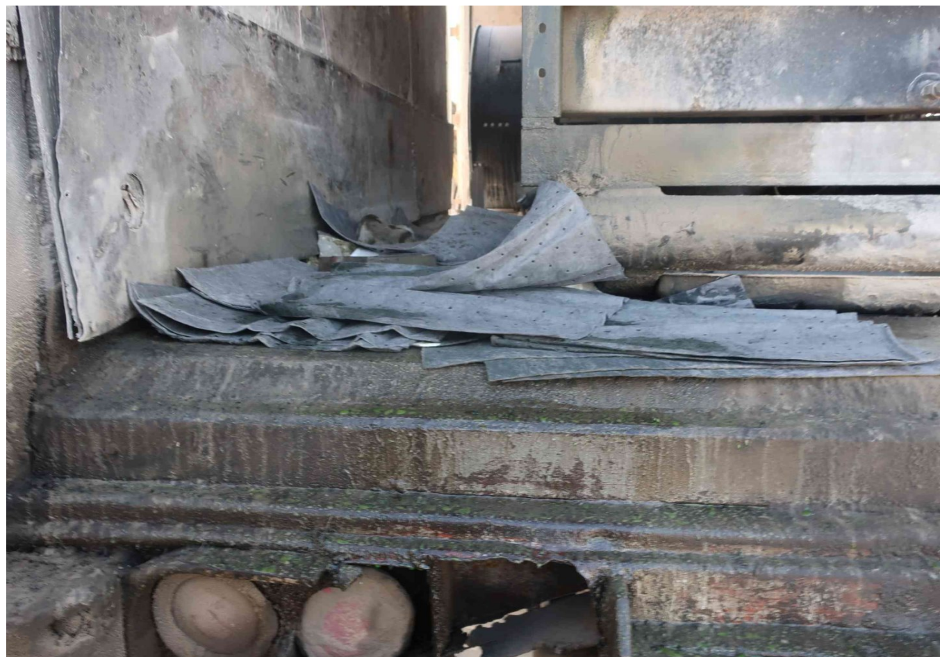
Figure 4 Glycol leaking out the back of the crusher generator trailer.
