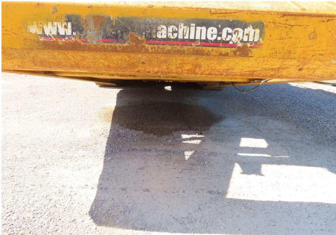
Figure 16 Hydrocarbon staining observed under the crusher. No drip tray was located under the parked equipment.
