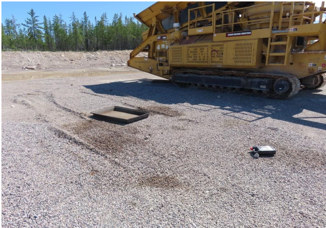
Figure 16 Hydrocarbon staining observed under the crusher. No drip tray was located under the parked equipment.
