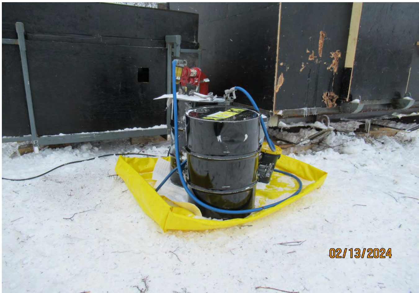
Figure 42 Fuel drums and the nozzle at the diamond drill are stored in secondary containment.
