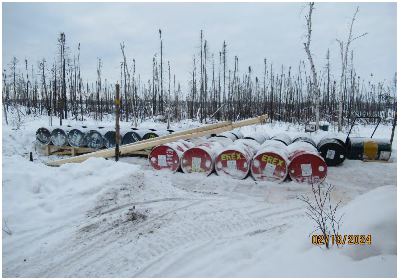
Figure 26 Gasoline drums have been placed in secondary containment and snowmobiles are being fueled overtop of this secondary containment structure.
