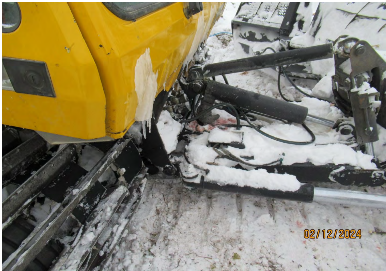
Figure 16 Personnel were wrapping fittings with absorbent matting to prevent further loss to the receiving environment. Persistent leaks must be repaired at the earliest opportunity.
