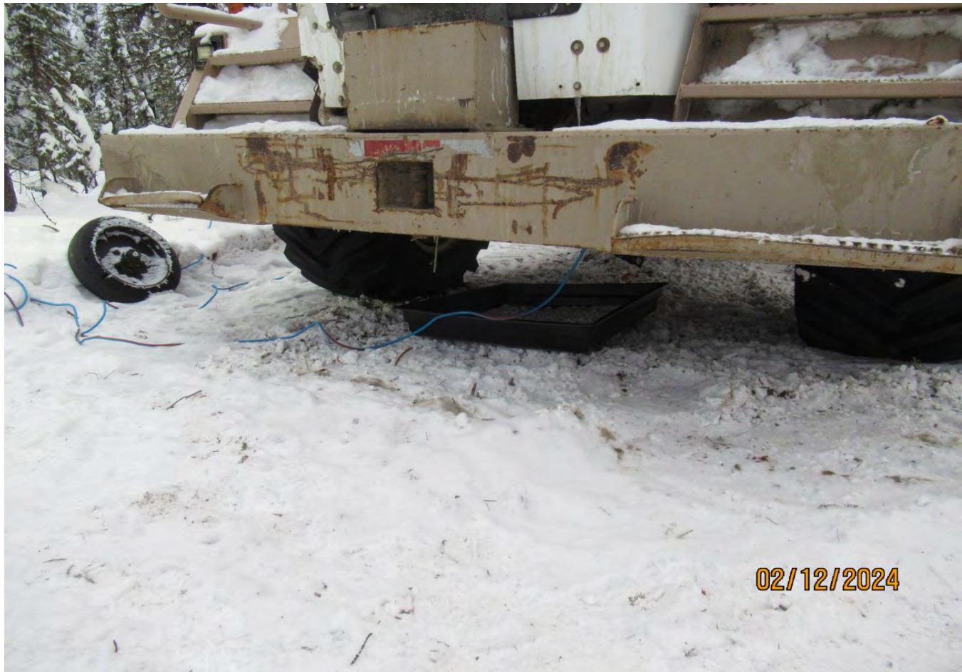
Figure 12 Drip tray was present below the one parked water truck.
