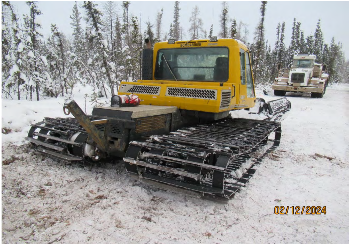
Figure 10 Snowcat parked adjacent to the portage. All parking areas on land must be watered in to protect the ground surface from damage and potential spills.
