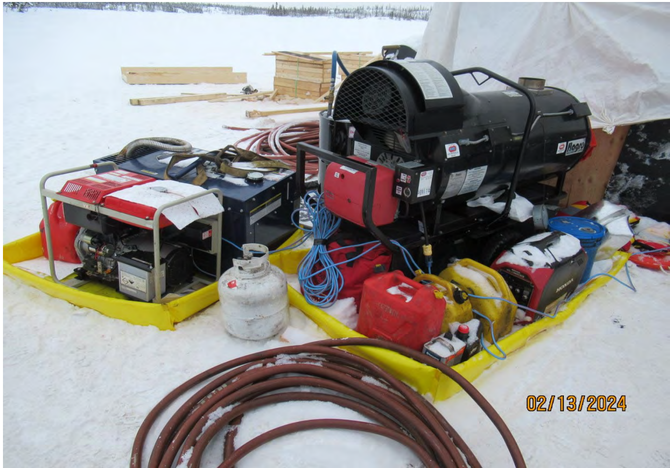
Figure 42 Fuel drums and the nozzle at the diamond drill are stored in secondary containment.
