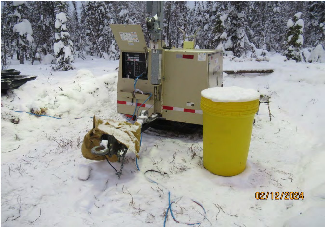
Figure 14 Light plant in the equipment laydown had a drip tray and a spill kit is present.
