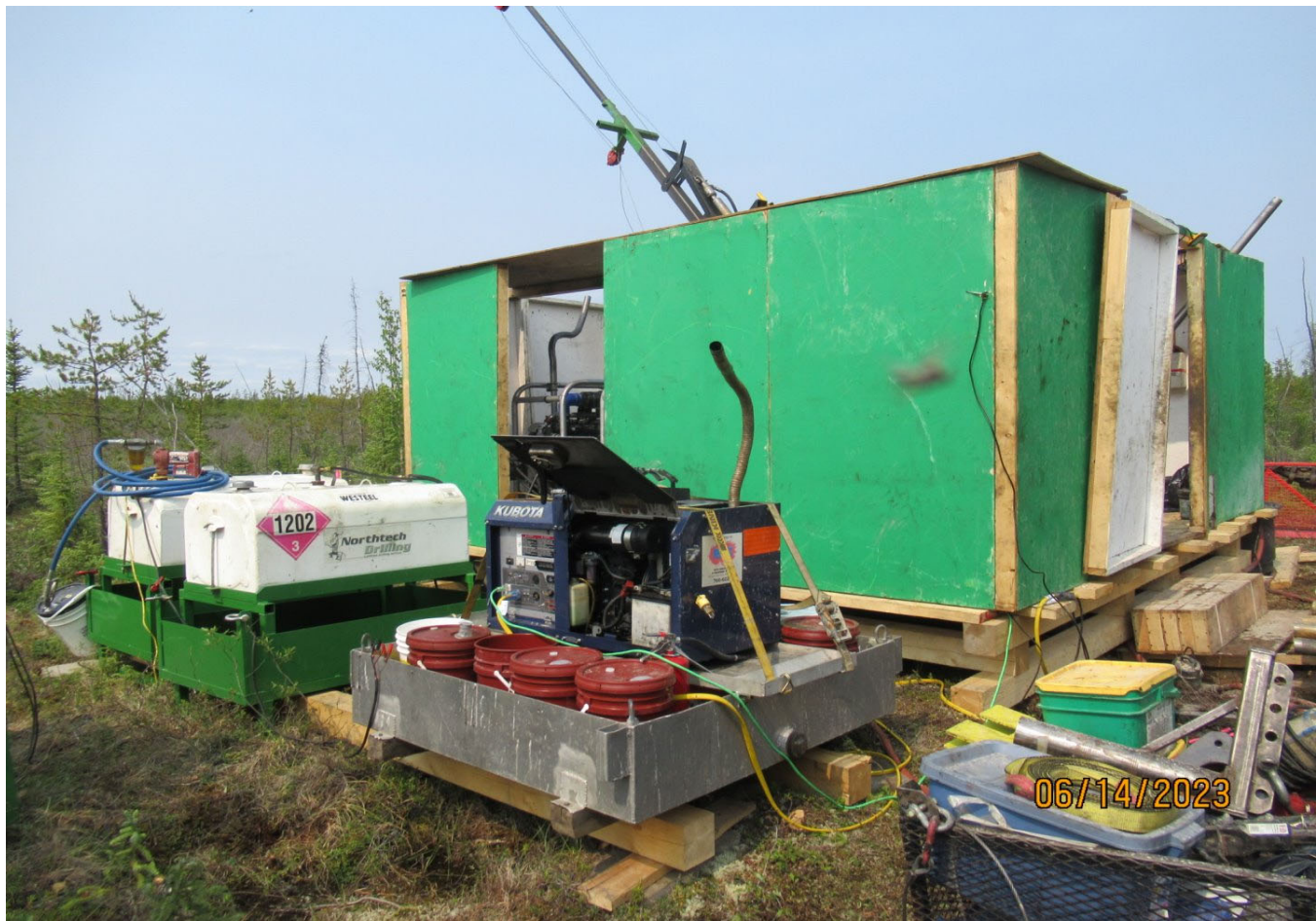
Figure 12 Top feed, double walled fuel tanks stored in tertiary containment at the Northtech drill. Generator and hydrocarbon pails are also being stored in secondary containment.
