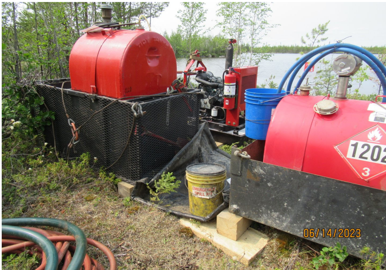
Figure 12 Top feed, double walled fuel tanks stored in tertiary containment at the Northtech drill. Generator and hydrocarbon pails are also being stored in secondary containment.
