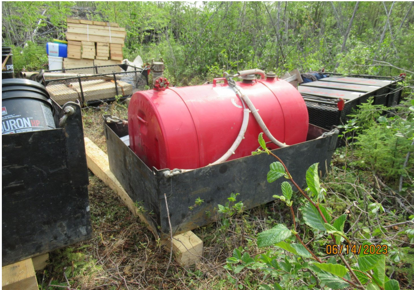
Figure 10 All of the Dorado fuel containers are being stored in secondary containment. Hydrocarbon absorbent matting must be placed on the water surface within the containment structure.
