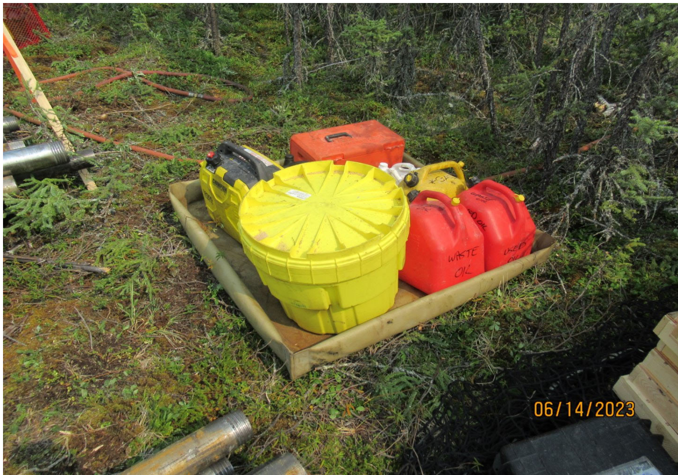
Figure 18 Hydrocarbon containers at the Northtech drill are stored in containment and spill response materials were present.
