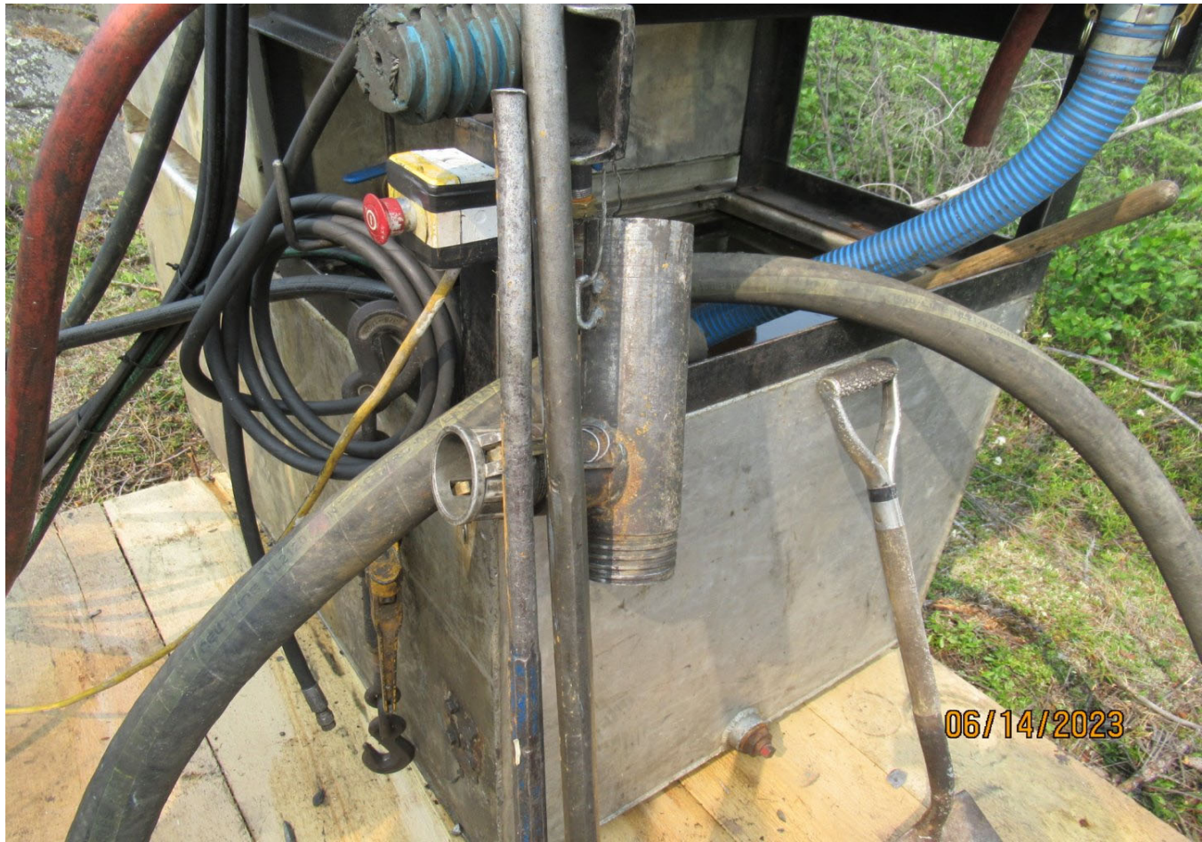
Figure 8 Water funnel is being used at the Dorado drill when pulling the core barrel. Water is directed back into the mud tank.
