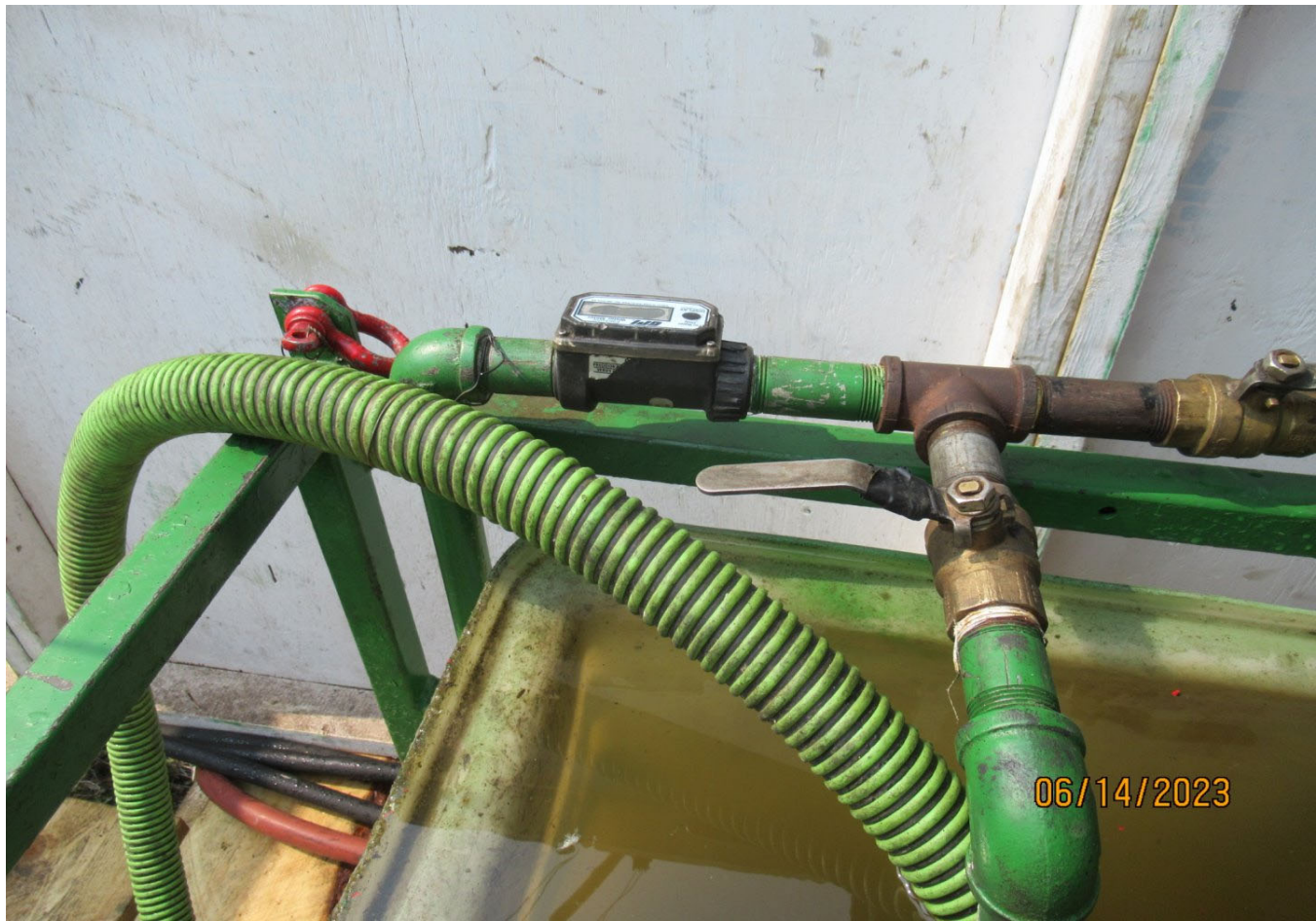
Figure 8 Water funnel is being used at the Dorado drill when pulling the core barrel. Water is directed back into the mud tank.
