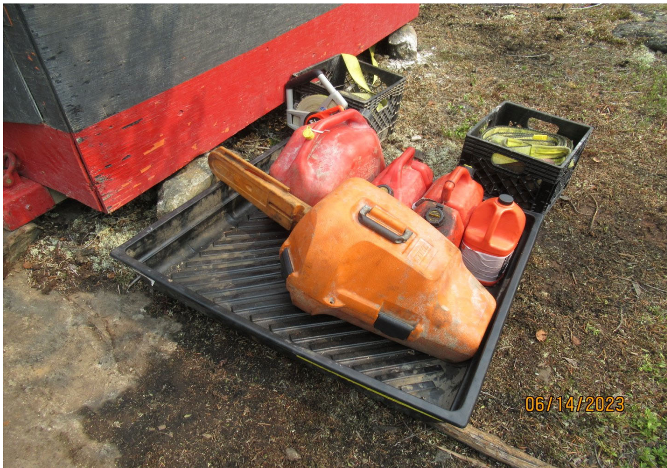
Figure 18 Hydrocarbon containers at the Northtech drill are stored in containment and spill response materials were present.
