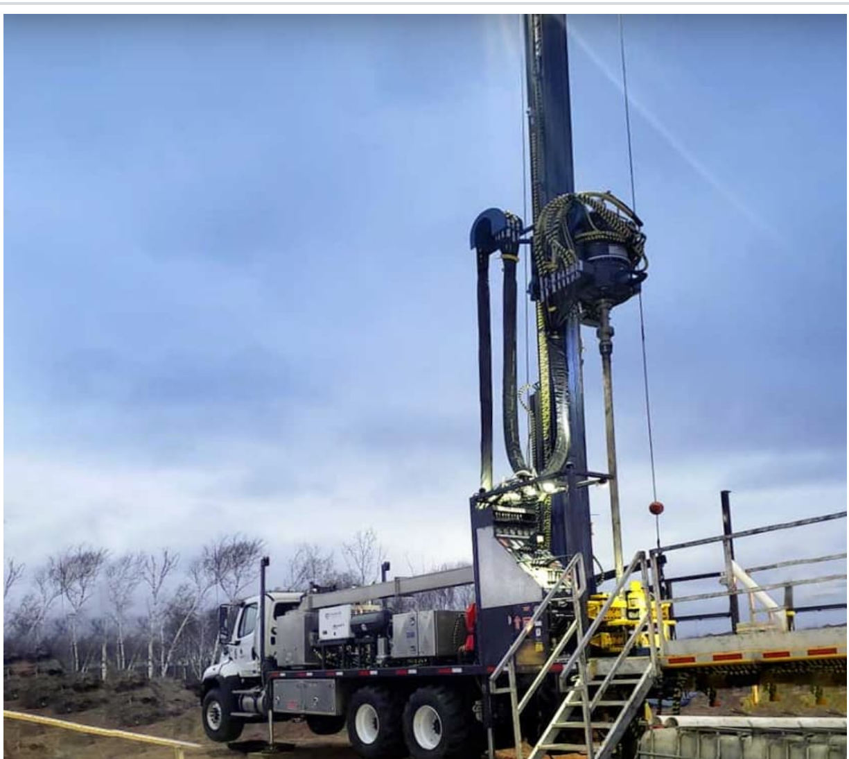
Figure 1. Gus Pech Brat-a-Sonic Truck Drill 50K Head Truck Mount Sonic
