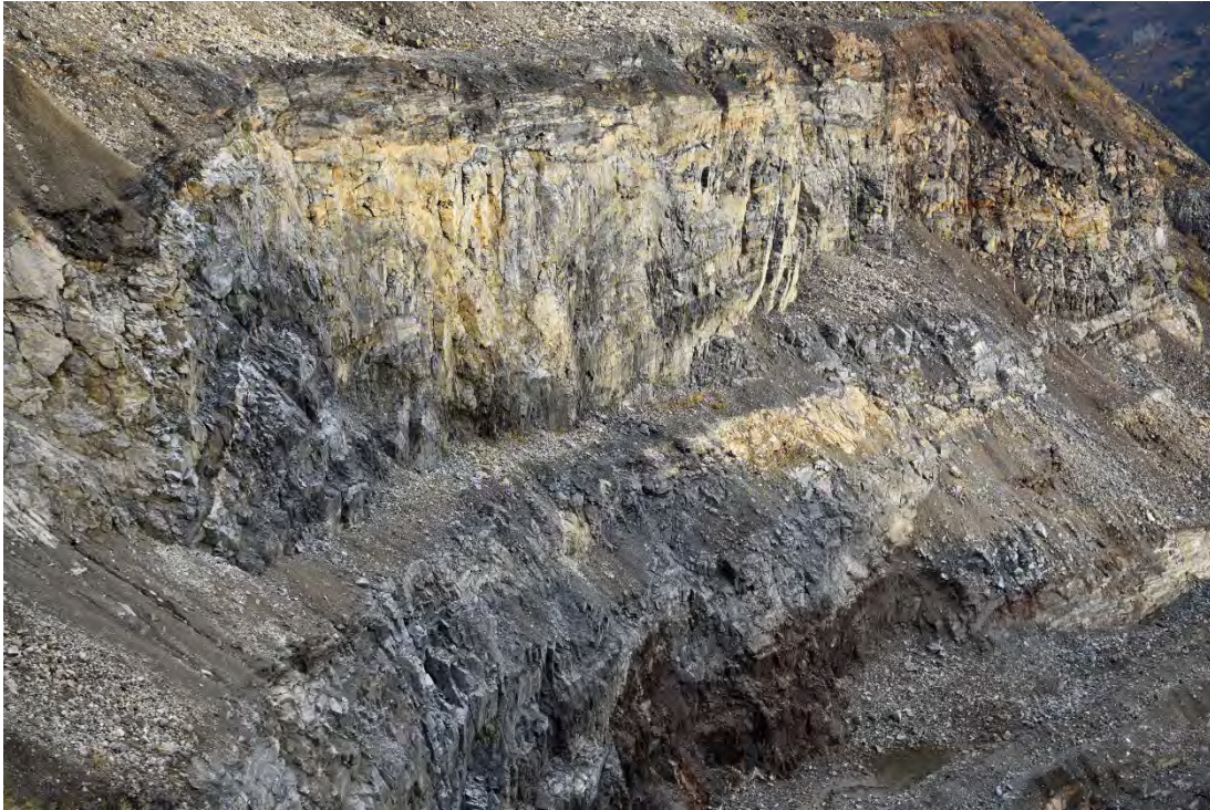
Photo 3: Middle benches of the NW wall of the Open Pit showing erosion and iron staining; note seepage from the face in the lower-right of the photo.
