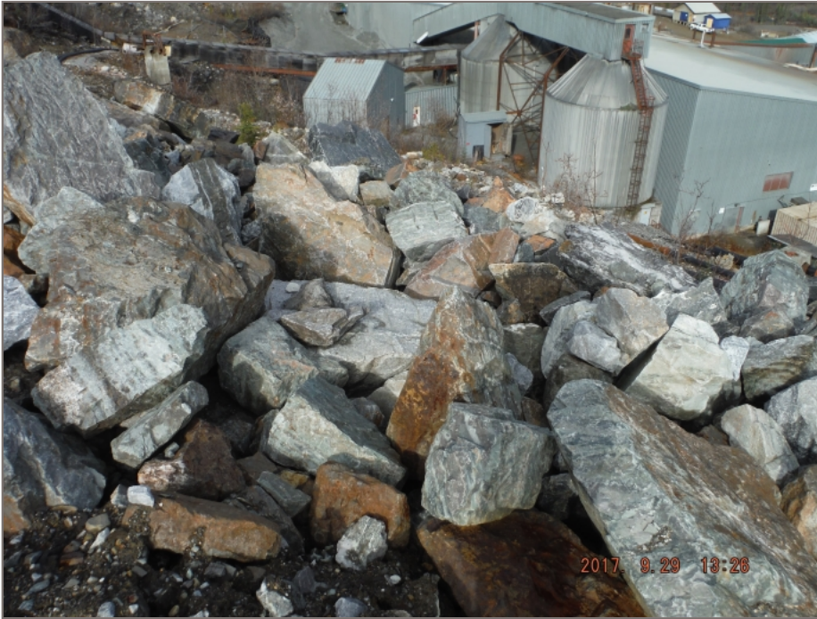
Photo 5: Ore stockpile dominated by skarnified swiss-cheese limestone including sulphide-rich pyrrhotite skarn. (September 29, 2017)
