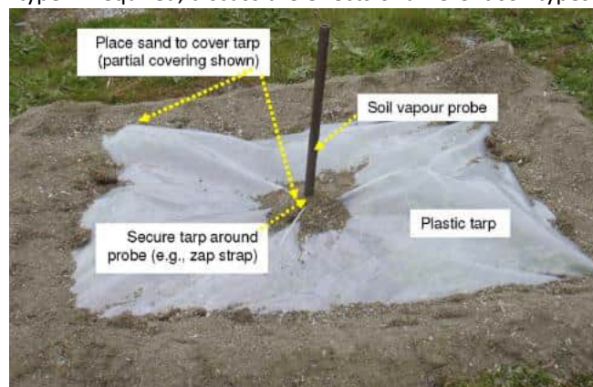
Figure 1. Secured surface seal around soil vapour probe.
