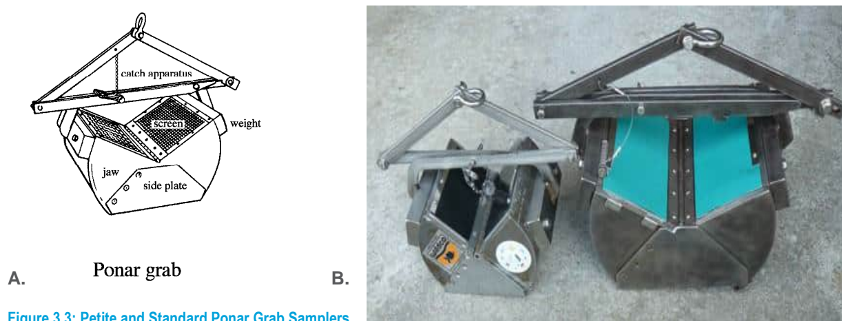
Figure 3.3: Petite and Standard Ponar Grab Samplers A. Schematic Diagram of a Ponar Grab Sampler; and, B. The two sizes of the Ponar Grab; the Petite (left) and the Standard (right).
