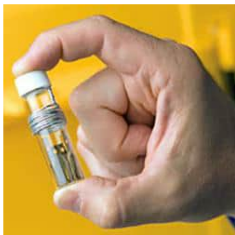
Figure 4.9: Example of a passive soil gas (PSG) sampler (left), and a schematic of passive sampling installations (right) (Figure adapted from: O'Neill, Harry, (2018) Passive Soil Gas Testing: Standard for Site Characterization).
