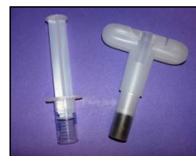
Figure 1. Terra-Core™ with soil plug and syringe samplers
