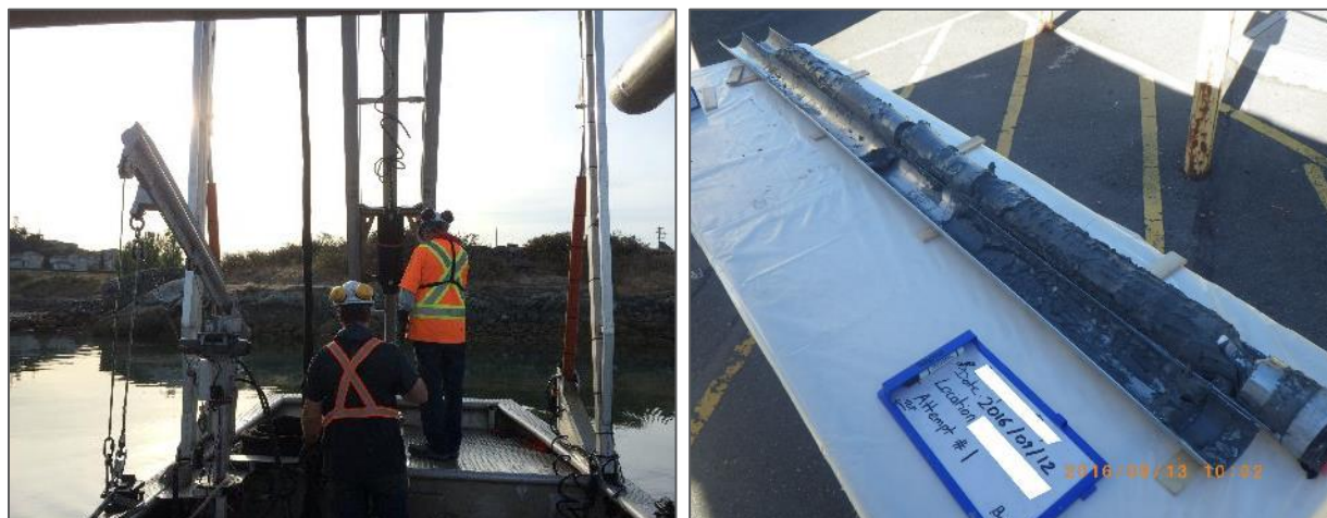
Figure 4.3: Photos of Vibracore Sampling and resultant Core.
