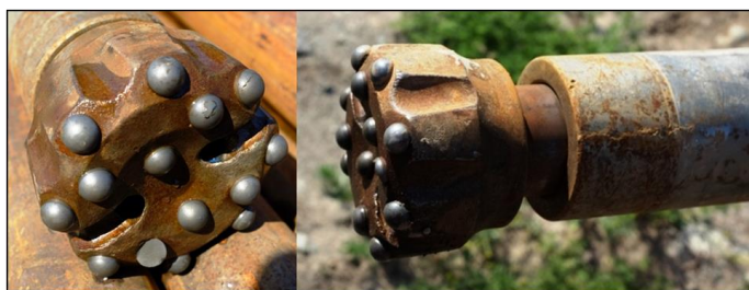
Figure 3.2: Air-operated down-the-hole hammer bit.
