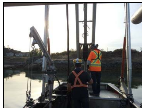
Figure 2: Vibracore sampling in marine environment
