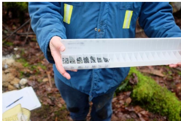
Figure 1. Chip tray used for sample storage.
