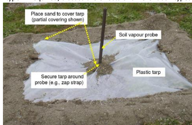
Figure 1. Secured surface seal around soil vapour probe.
