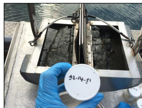
Figure 4: Ponar grab sampler full of sediment following retrieval.
