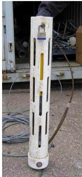
Figure C-14. An example of a slotted deployment tube. The figure on the right shows the bar across the top that both prevents access to the sonde and sensors and helps support the sonde. Photos: Frank van der Have
