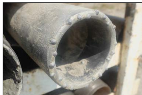
Figure 3. Vibrasonic drill bit.
