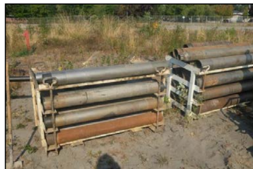
Figure 2. Vibrasonic core barrels.
