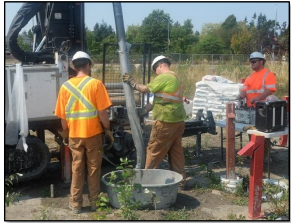
Figure 4. Recovery of Vibrasonic core.
