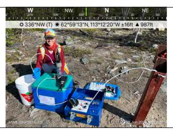
Magda Celejewski setting up groundwater monitoring and sampling equipment at well MW6 (SNP2016-8d).
