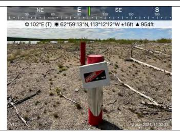
Vibrating wire thermistor VT2 datalogger .
