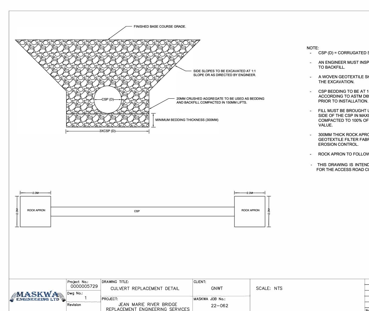
CSP (D) = CORRUGATED STEEL PIPE DIAMETER.
