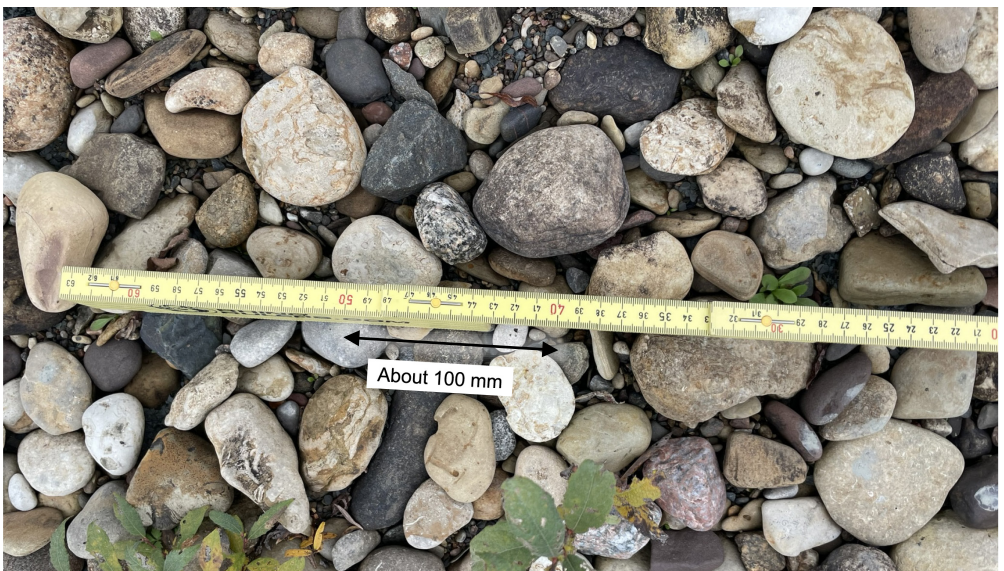
Photograph 8: The gravel bar downstream of the bridge ( D_{50} about 100 mm).
