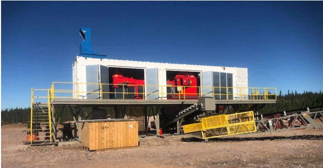
Figure 6: Ore Sorting Plant initial installation at Nechalacho North T Bulk Sample Project
