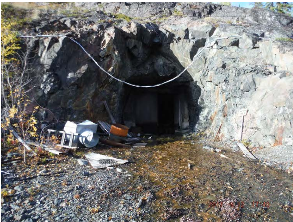
Photo 25 Northrim Mine- Station NO-9: Water drainage from adit, too shallow to sample (<2 cm) in areas without rock overhang (downstream sample collected)
