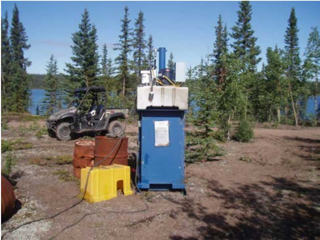
Hydraulic drum crusher, to light to crush the drums on site.
