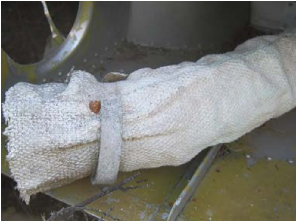
Photo 44: Suspected asbestos containing material surrounding the fuel pipe inside the plane fuselage at SA-DA-20, Sawmill Bay ↑
