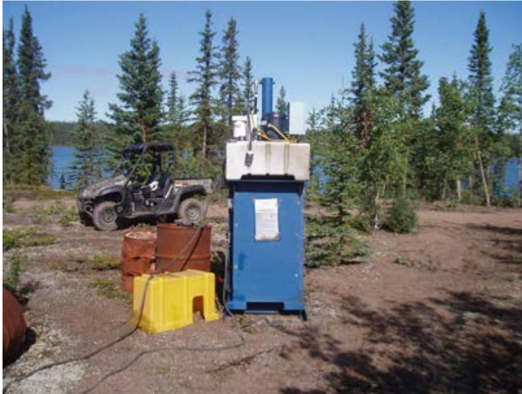
Photo 3: All drum crushing occurred at Sawmill Bay. Hydraulic drum crusher not strong enough ↑
