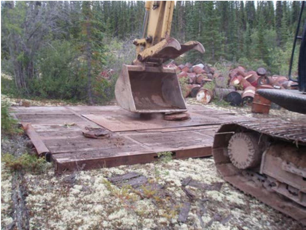
Trial run on crushing drums with the Cat320C.
