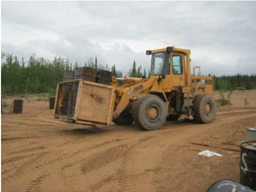
Using the front-end loader to move drums to the wash site. Box is lined with spill pads.
