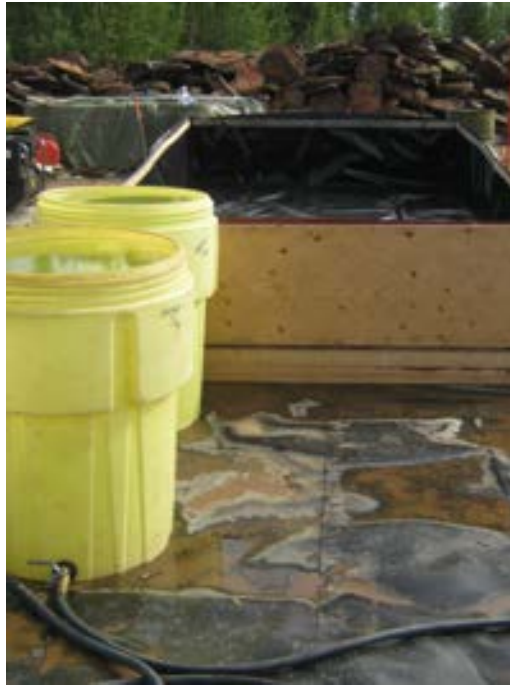
The lined box will house the drum holder for washing. The yellow tanks will house absorbant booms to remove hydrocarbons. The wash water will be cycled through the system.
