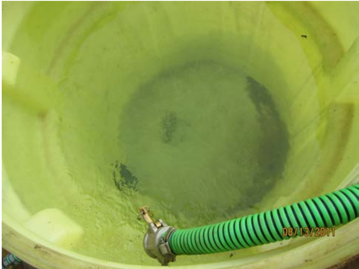
Treated water pumped into this overpack for 'hotsie' use. The water is used for cleaning drums using the pressure washer.
