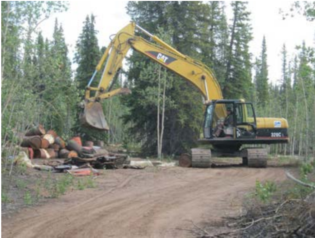
Using the excavator to crush drums. There was no labourer helping the excavator, thus the steel safety shield is not in use.
