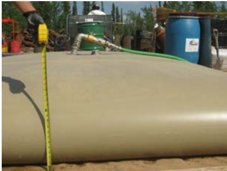
Holding bladder at approximately 85% capacity
