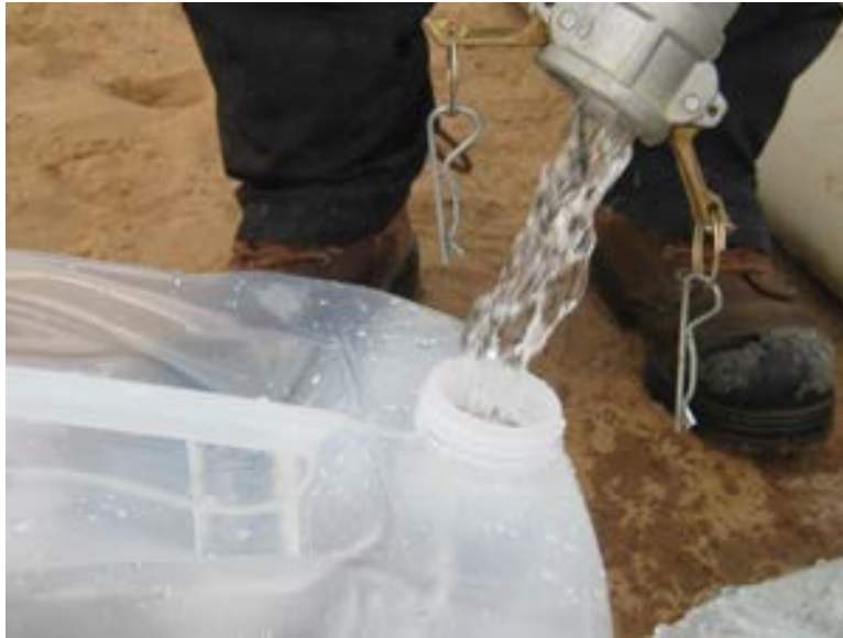
Treated liquid being collected for sample SB-W-1. Note that the three 20 litre jugs are required for toxicity testing. This hose normally inputs into the holding bladder.
