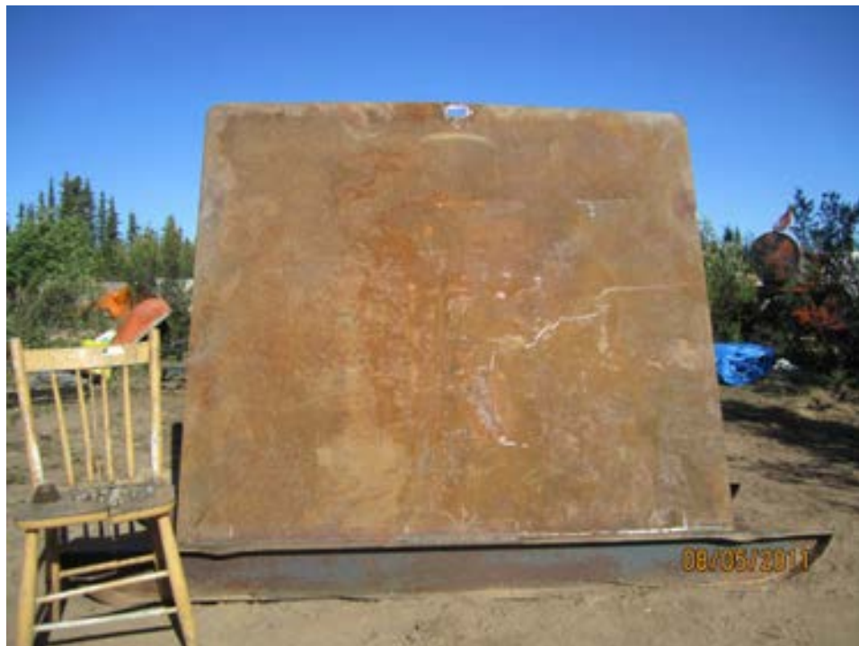
The protective shield to be used during crushing activities. It measures 6' x 6'
