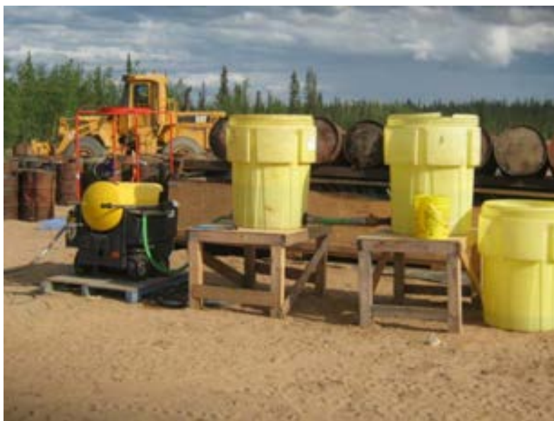
The 'hotsie' pressure washer system. Water will be recycled through the system. Note there will be absorbent diapers used to collect oil from the washed drums.
