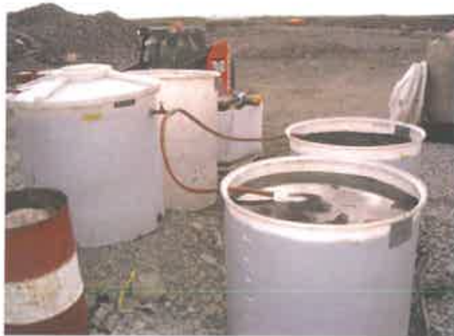
Figure 8 - AEL Setup of the Activated Carbon Tanks
