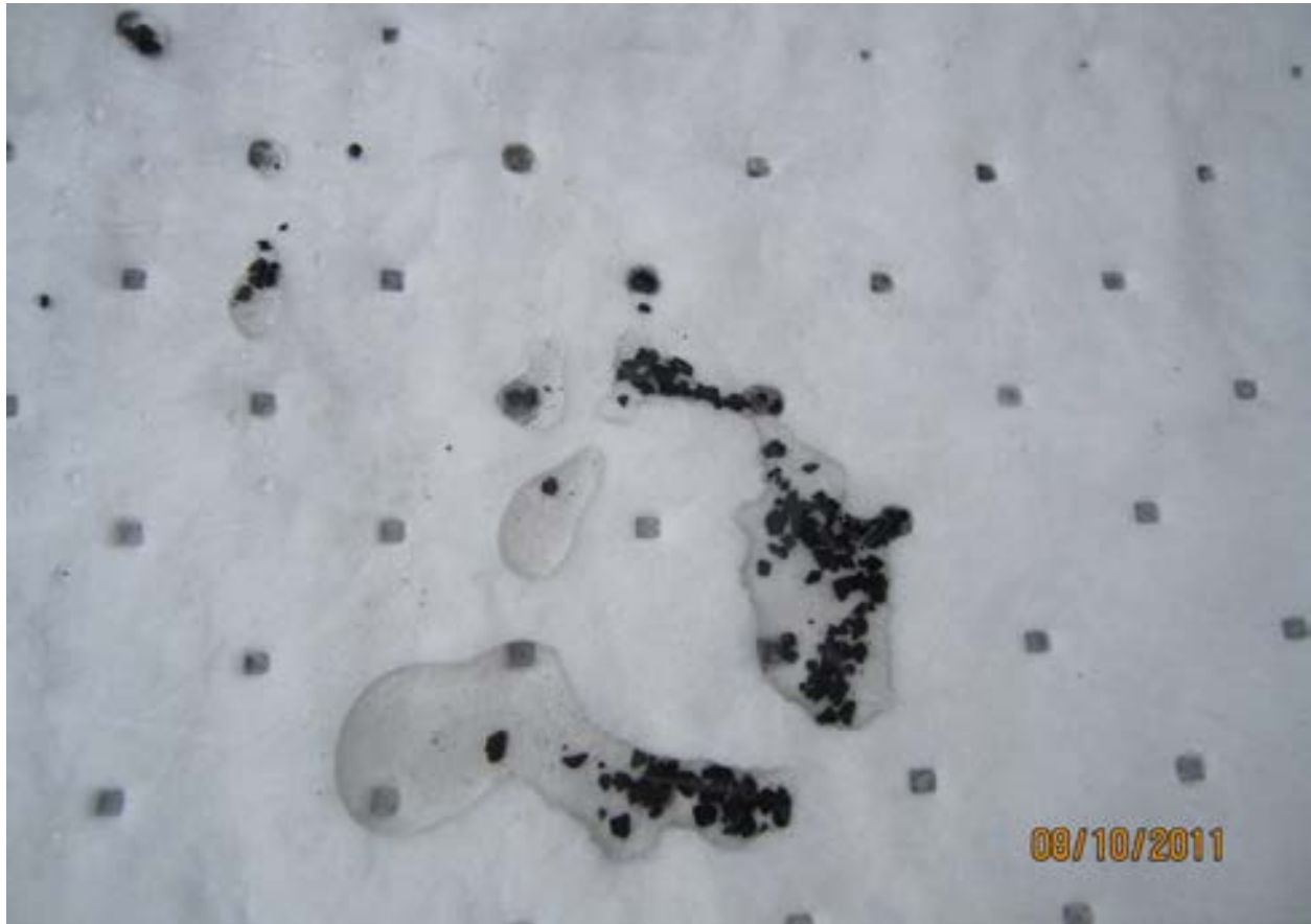
Activated carbon and water on an oil absorbent diaper. Note the beading water. Activated carbon soaking overnight for replacement tomorrow.
