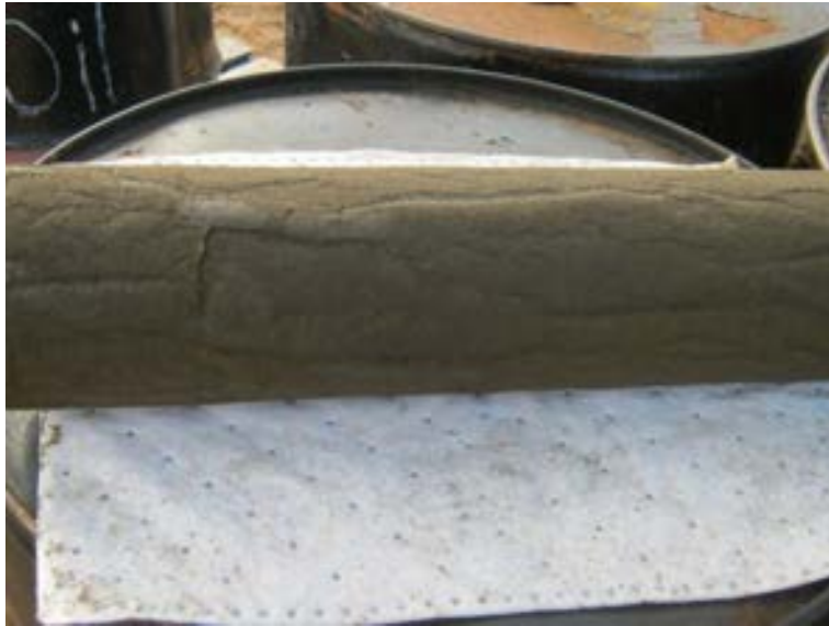
A sediment filter changed out. The sediment filter is housed in the blue box, immediately after the oil-water separator.
