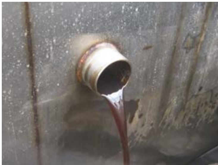
The skimmed oil pouring into a separate compartment
