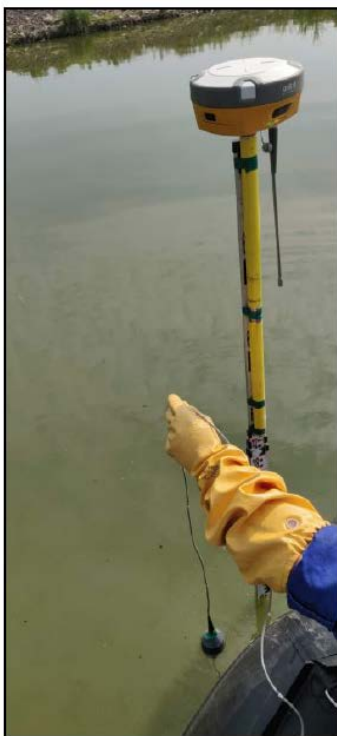
Figure 1.5: Sludge and liner measurement using sludge gun, GNSS and metered survey rod (Hydrasurvey, 2019)
