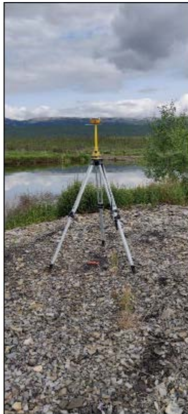
Figure 1.4: GNSS base station setup (Hydrasurvey, 2019)
