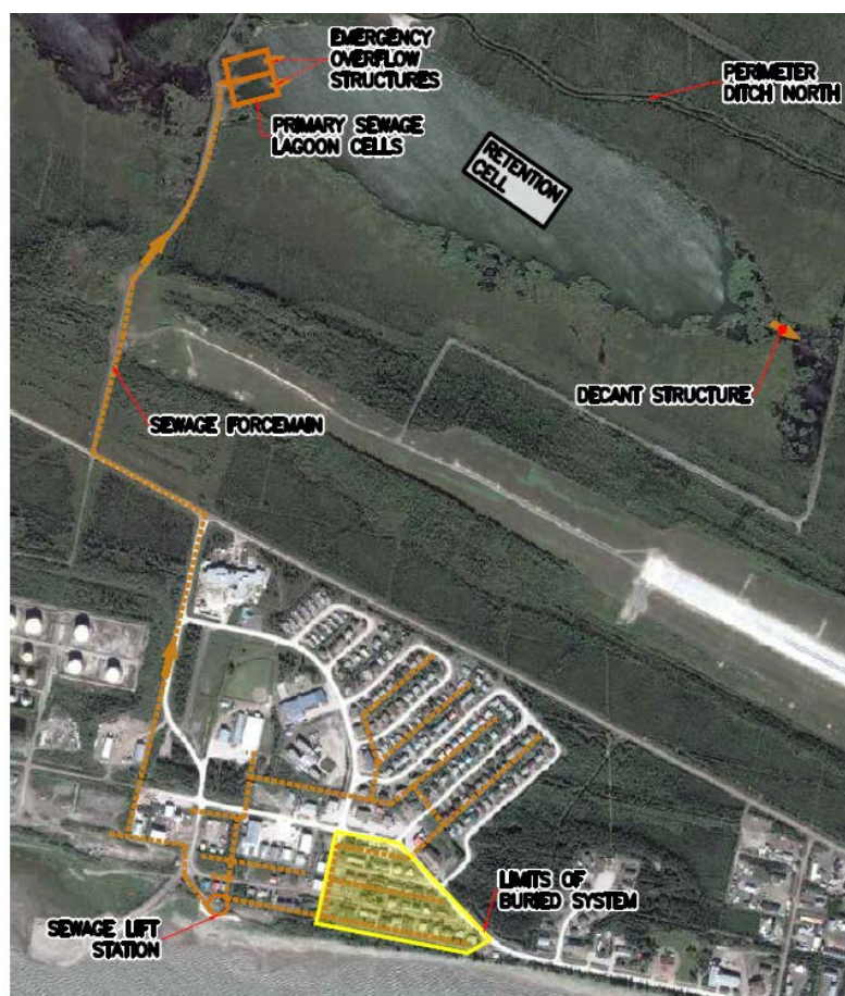
Figure 1.2: Town of Norman Wells Wastewater Flow Sequence
