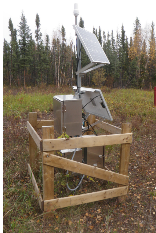
An Enbridge earth station with solar panels, batteries, a data logger and antenna. Earth stations are used in remote areas to power slope monitoring instruments which measure and record ground movement.
