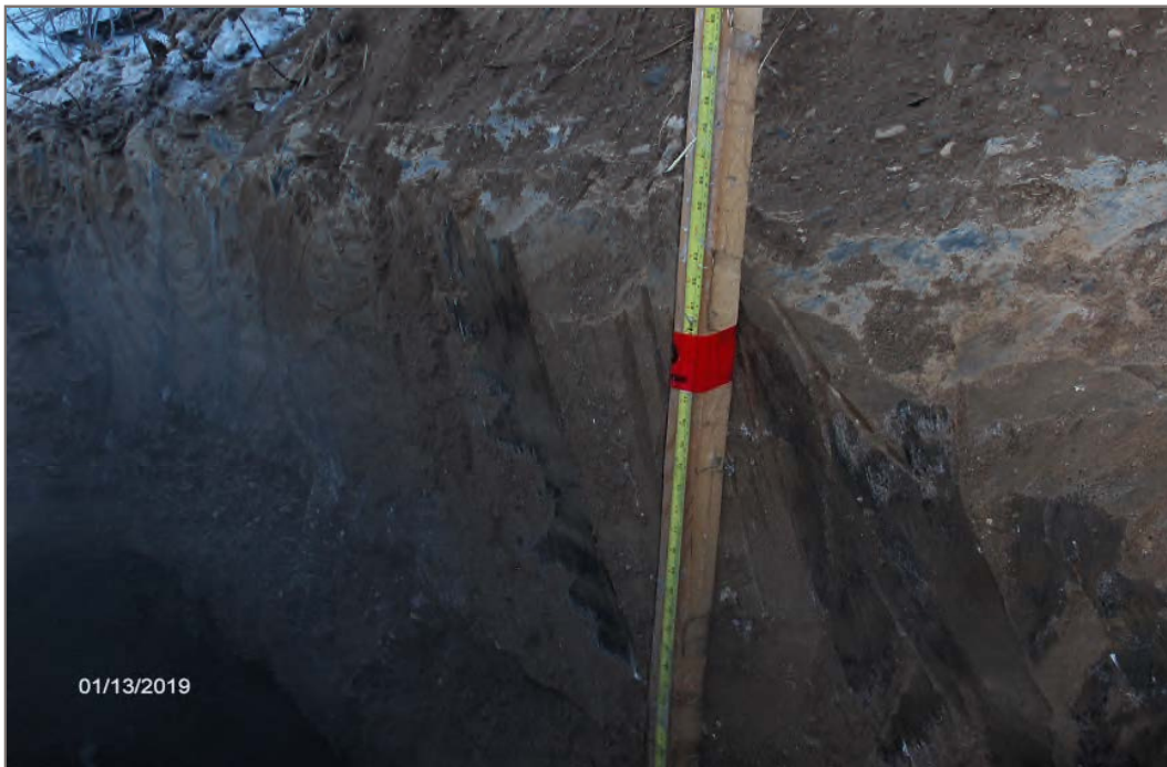
Photo 12: Prospect 1, Testpit 8. Sand, silty underlain by gravel starting at about 1.5 m depth.
