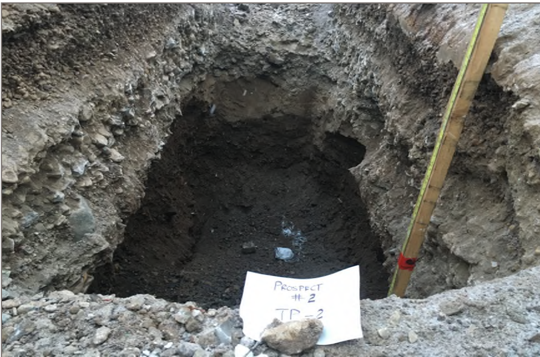
Photo 14: Prospect 2, Testpit 2. Boulder can be seen in left wall.
