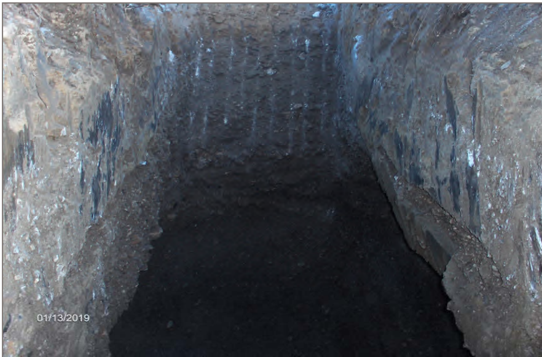
Photo 8: Prospect 1, Testpit 4. Gravel at approximately 1.0 m depth underlain by gravelly sand.
