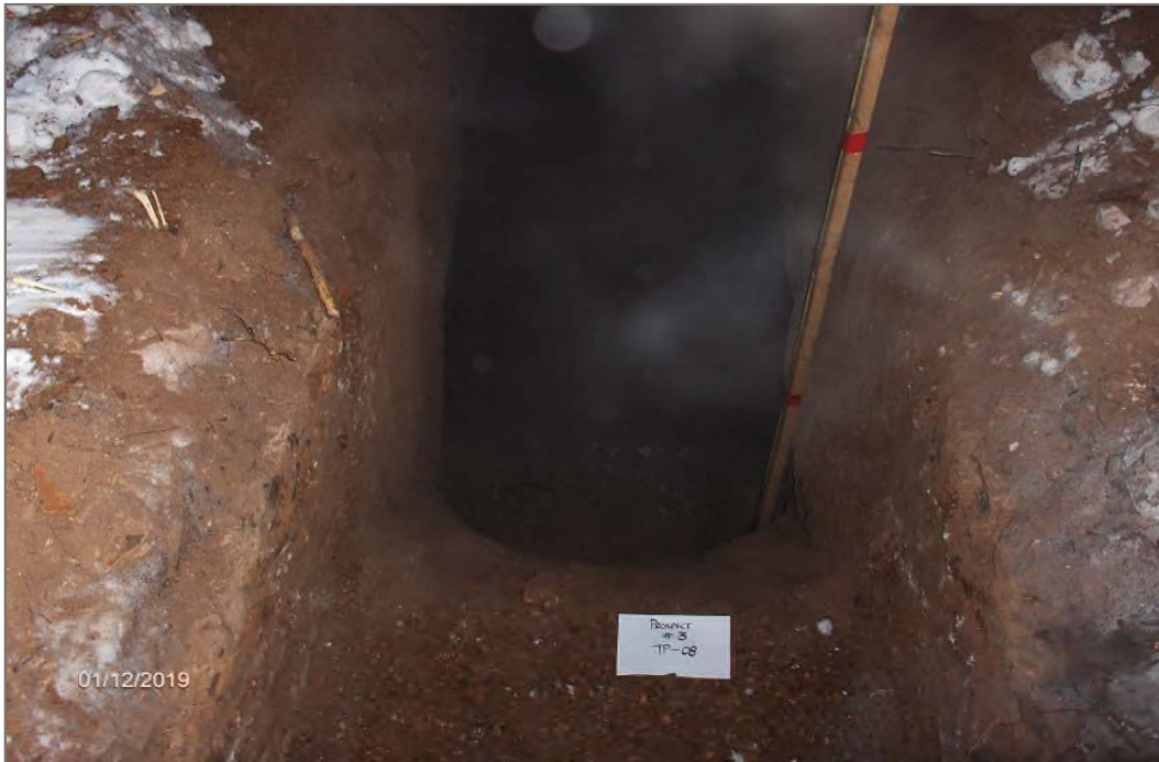
Photo 29: Prospect 3, Testpit 8. Gravel and sand from 0.5 m to 4.5 m depth.
