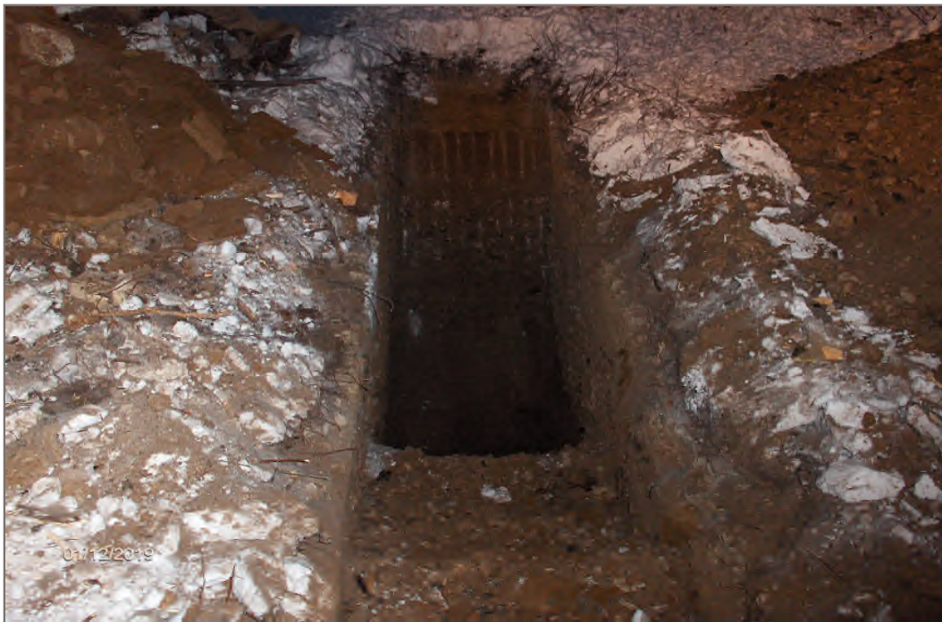
Photo 30: Prospect 3, Testpit 9. Gravel, sandy and sand from 1.0 m to 4.0 m.
