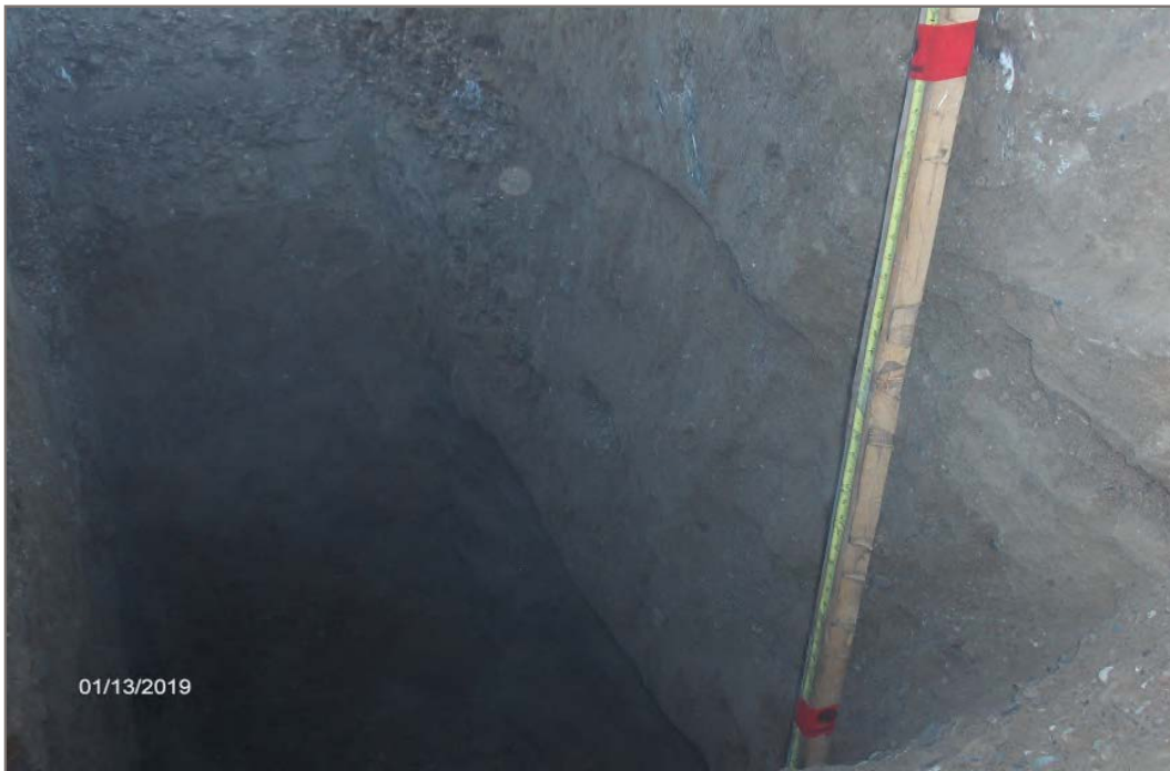
Photo 10: Prospect 1, Testpit 6. Alternating layers of sandy gravel and silty sand.
