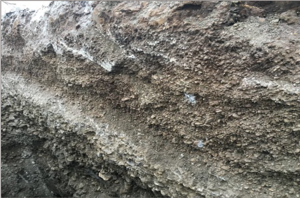
Photo 17: Prospect 2, Testpit 3. Gravel, sandy from 0.3 m to 4.2 m depth.
