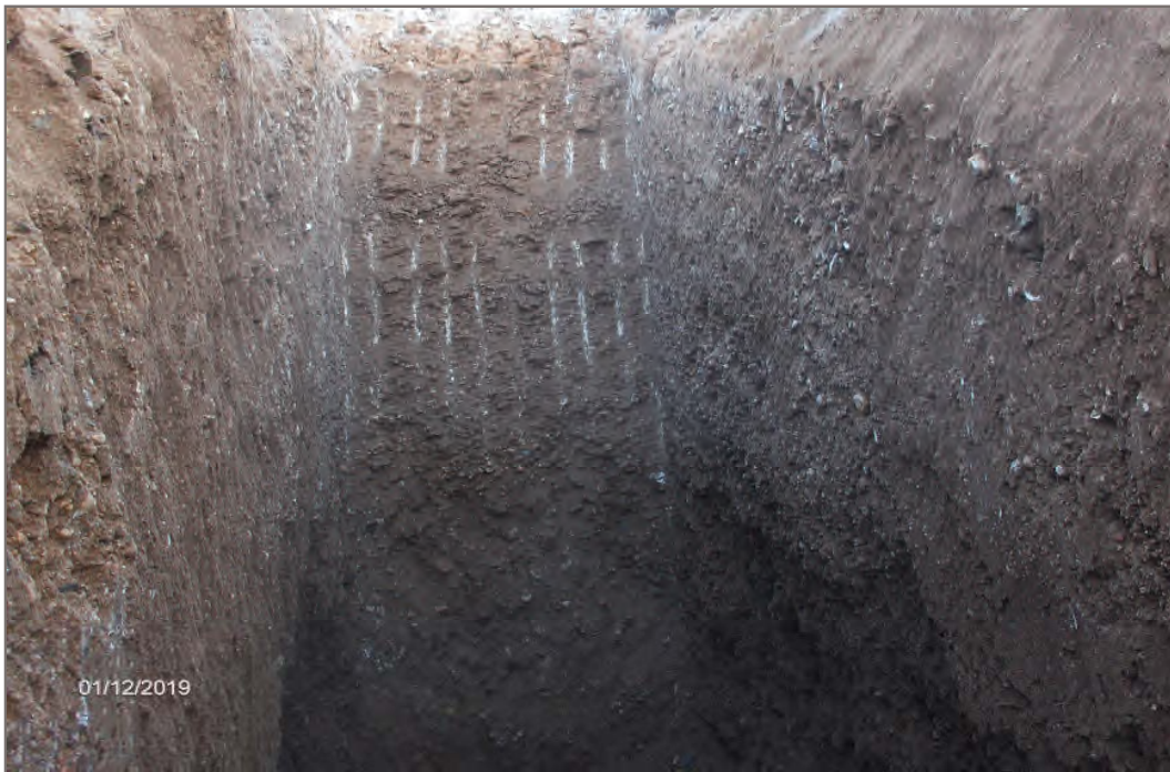
Photo 26: Prospect 3, Testpit 5. Gravel, sandy from 0.4 m to 4.0 m depth.
