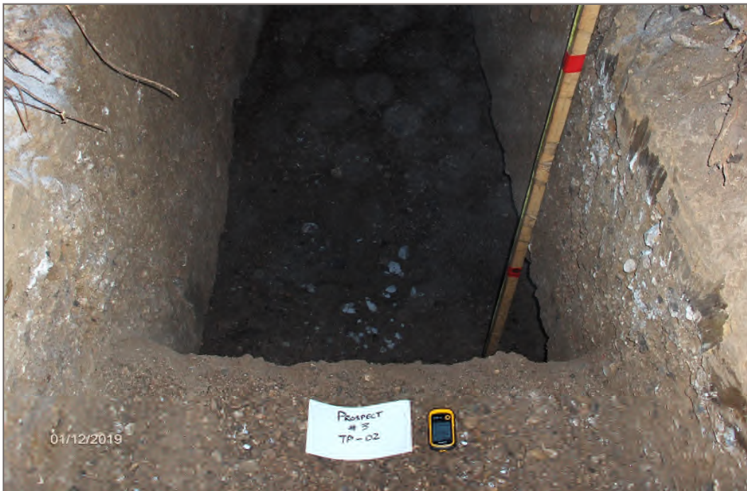
Photo 22: Prospect 3, Testpit 2. Gravel, sandy from 0.3 m to 4.0 m depth.
