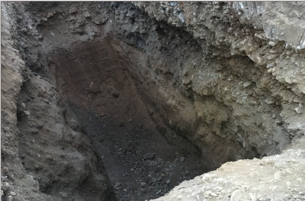
Photo 20: Prospect 3, Testpit 1. Gravel, sandy from 0.4 m to 2.0 m depth.
