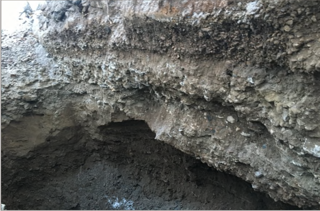
Photo 15: Prospect 2, Testpit 2. Gravel from 0.8 m to 1.5 m depth.
