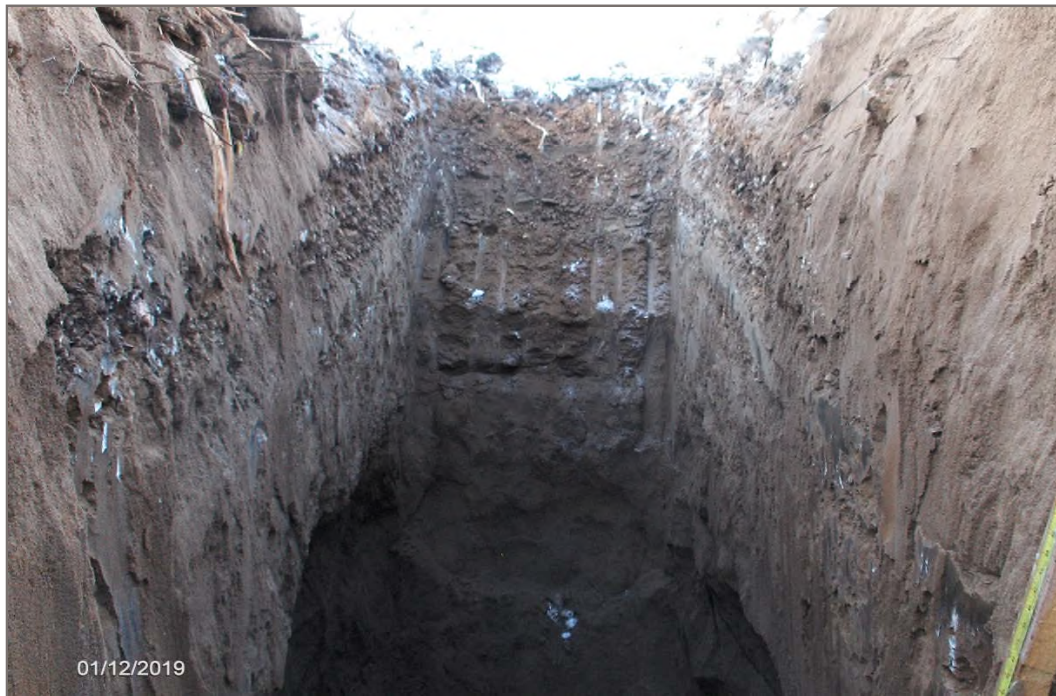
Photo 28: Prospect 3, Testpit 7. Gravel, sandy from 0.6 m to 1.5 and sand, gravelly from 1.5 m to 3.5 m depth.
