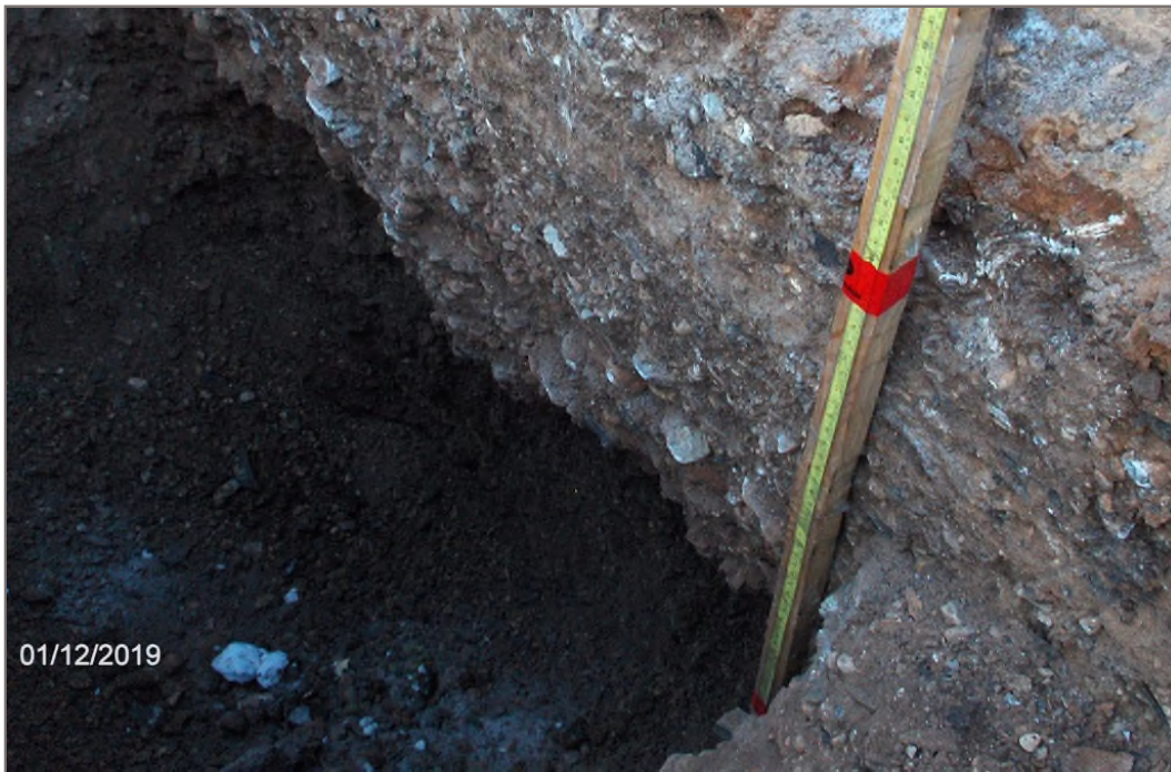
Photo 24: Prospect 3, Testpit 3. Coarse-grained materials from 0.5 m to 1.6 m depth.
