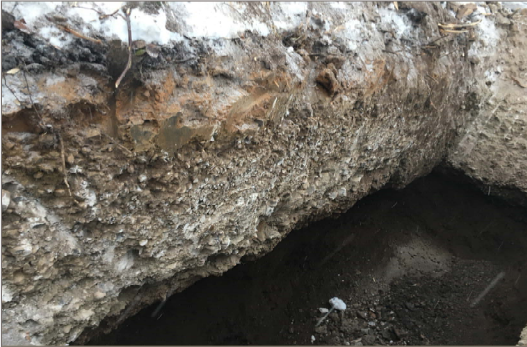
Photo 19: Prospect 2, Testpit 4. Gravel, sandy from 0.3 m to 1.2 m depth.
