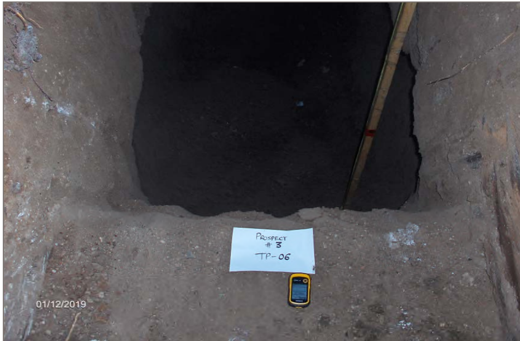
Photo 27: Prospect 3, Testpit 6. Sand and gravel from 0.5 m to 4.5 m depth.
