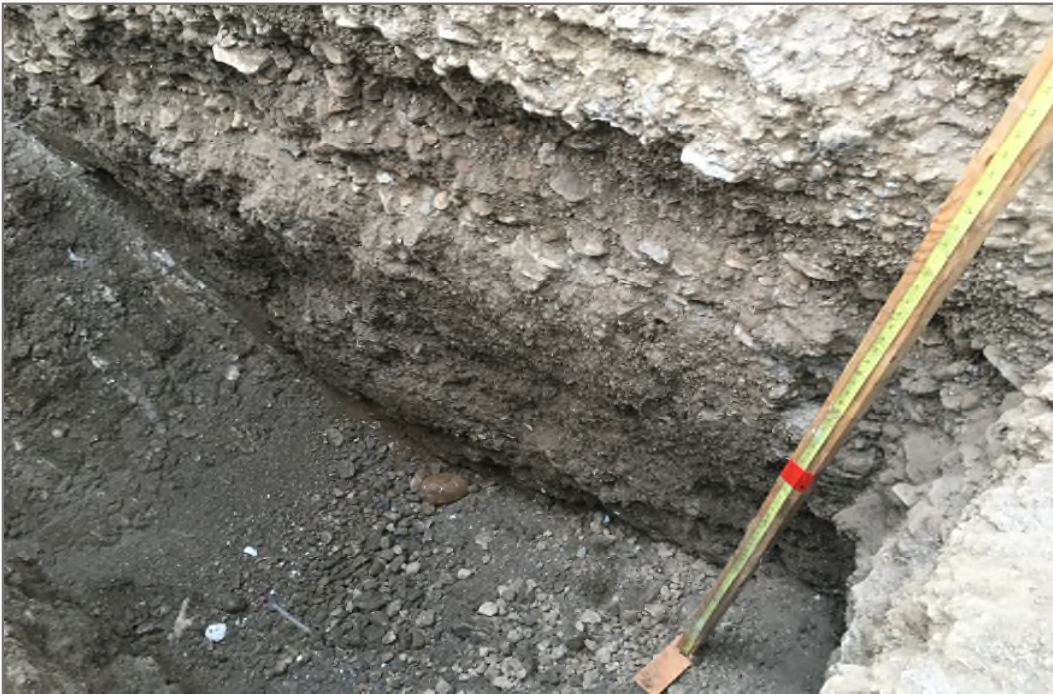
Photo 16: Prospect 2, Testpit 3. Gravel, sandy from 0.3 m to 4.2 m depth.
