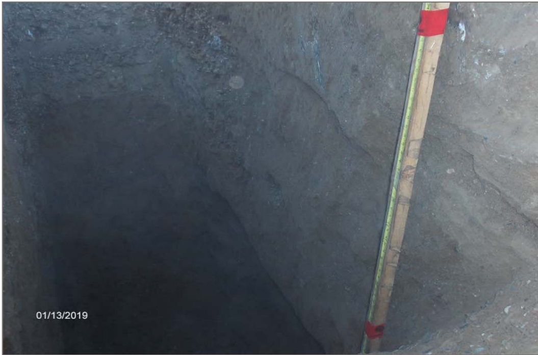
Photo 9: Prospect 1, Testpit 5. Alternating layers of sandy gravel and silty sand.
