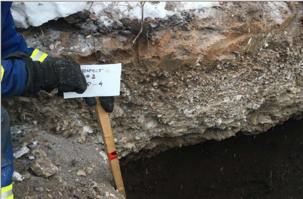
Photo 18: Prospect 2, Testpit 4. Gravel, sandy from 0.3 m to 1.2 m depth.
