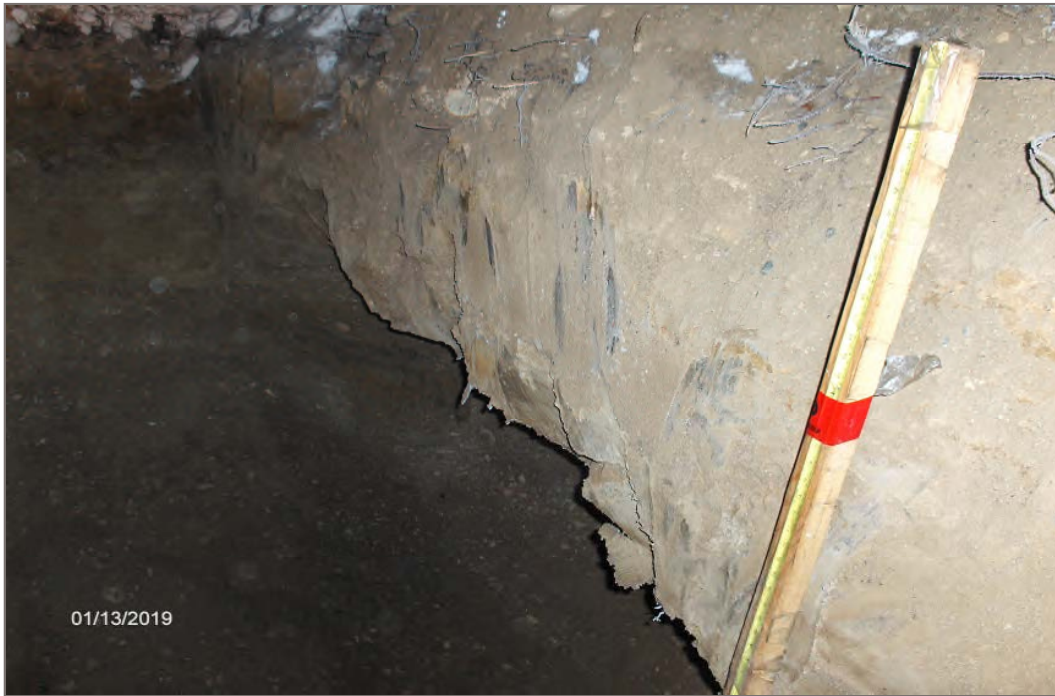
Photo 7: Prospect 1, Testpit 3. Sand, silty underlain by topsoil.
