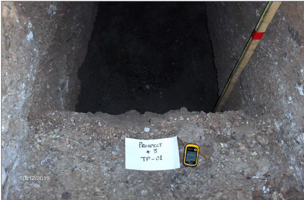
Photo 21: Prospect 3, Testpit 1. Gravel, sandy from 0.4 m to 4.2 m depth.
