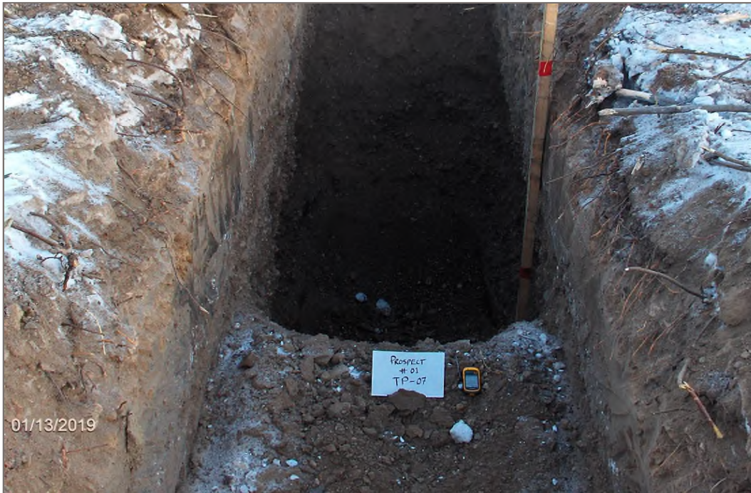
Photo 11: Prospect 1, Testpit 7. Sand, silty underlain by topsoil and gravels to about 1.0 m depth.
