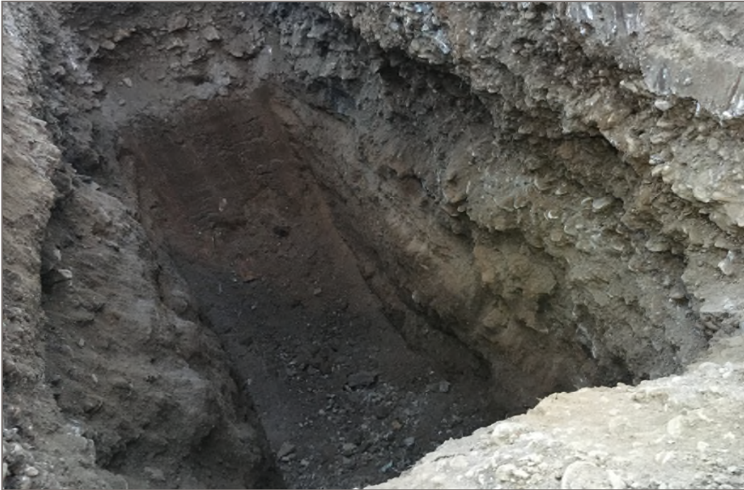
Photo 13: Prospect 2, Testpit 1. Gravel, sandy from 0.4 m to 2.0 m depth.
