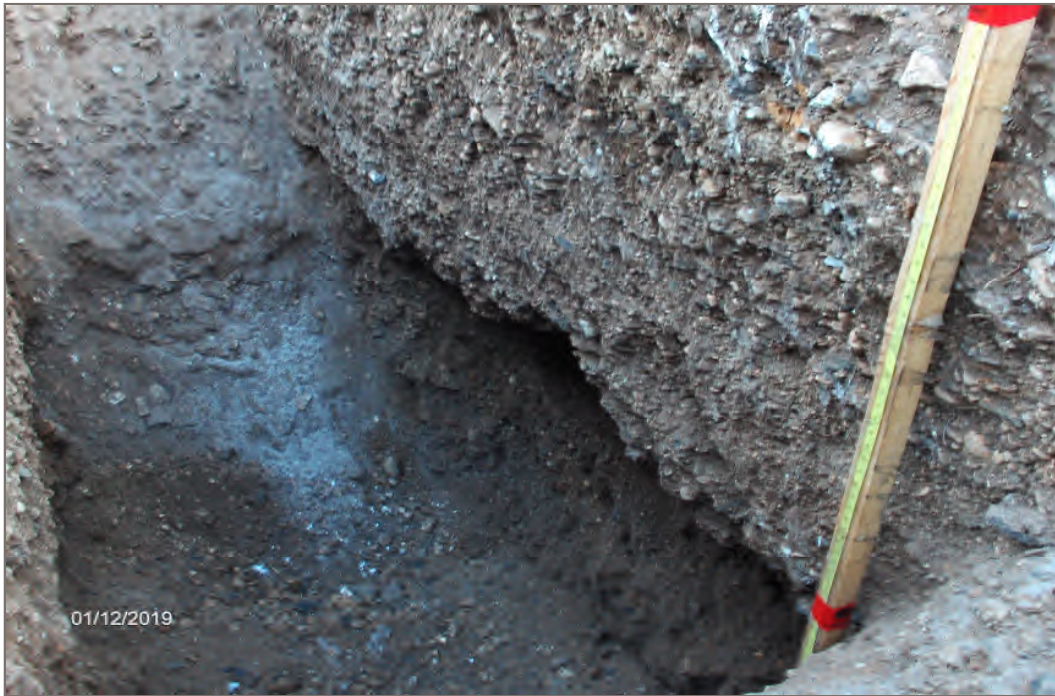
Photo 25: Prospect 3, Testpit 4. Gravel from 0.6 m to 4.5 m depth.
