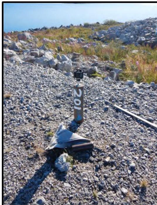
Photo D30: Survey prism monument (survey marker) along the downstream crest.
