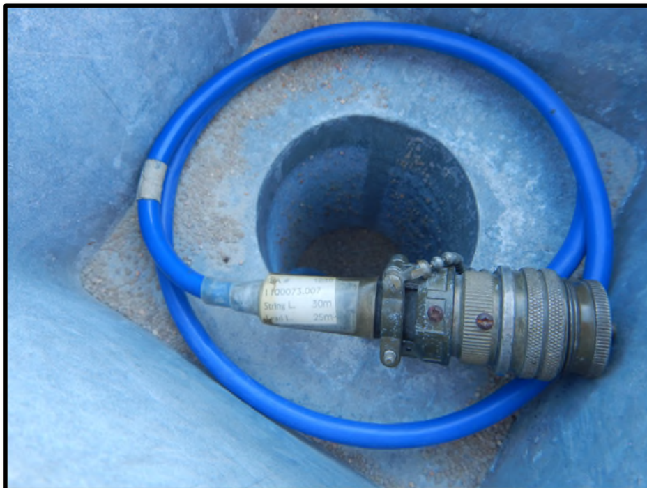
Photo D38: Ground temperature cable connector within protective instrumentation housing showing in Photo D37.
