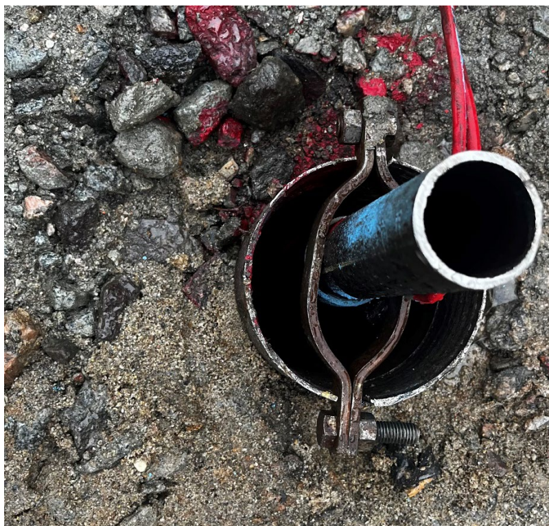
Photo 10: Borehole collar with installed Total Earth Pressure Cell and Piezometer into the 9080 Level Drift.
