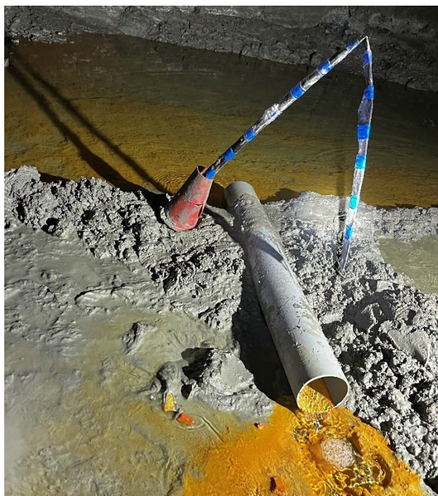
Photo 3: California Pipe used to measure Flow Rate at 9080 Bulkhead.
