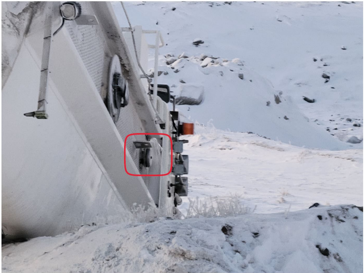
Figure 3: Flow of diesel from top air vent of overturned truck.
